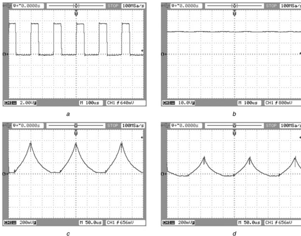
**Fig. 10** Typical waveforms in DCM
