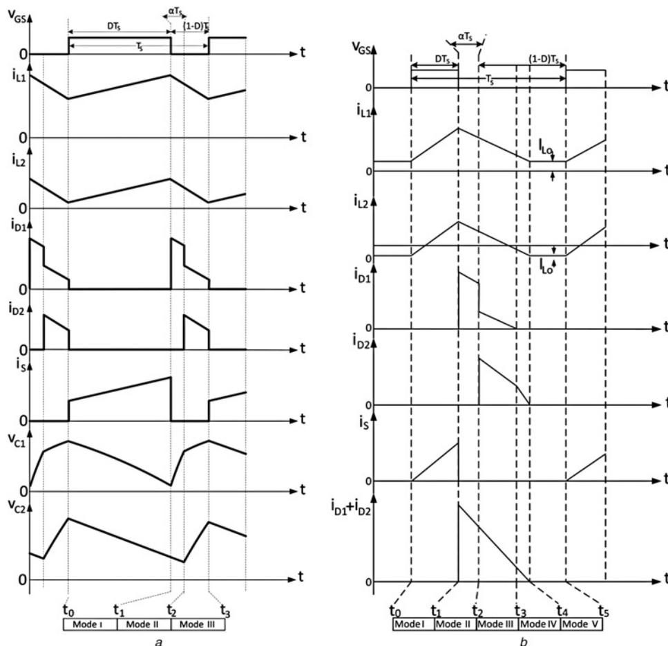
Fig. 2 Typical waveforms of the proposed converter
