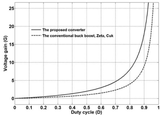
Fig. 4 Voltage gains of the proposed converter and Cuk converter in CCM operation
