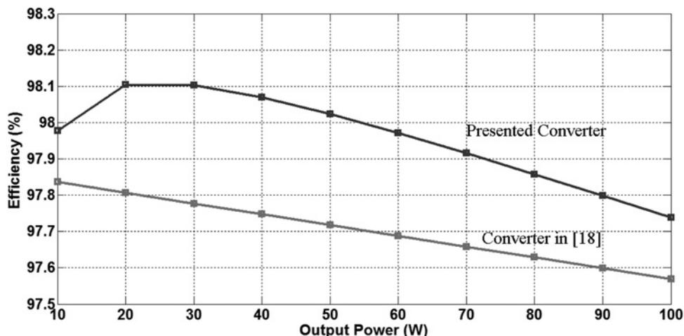
Fig. 8 Efficiency of the presented converter for various output powers
