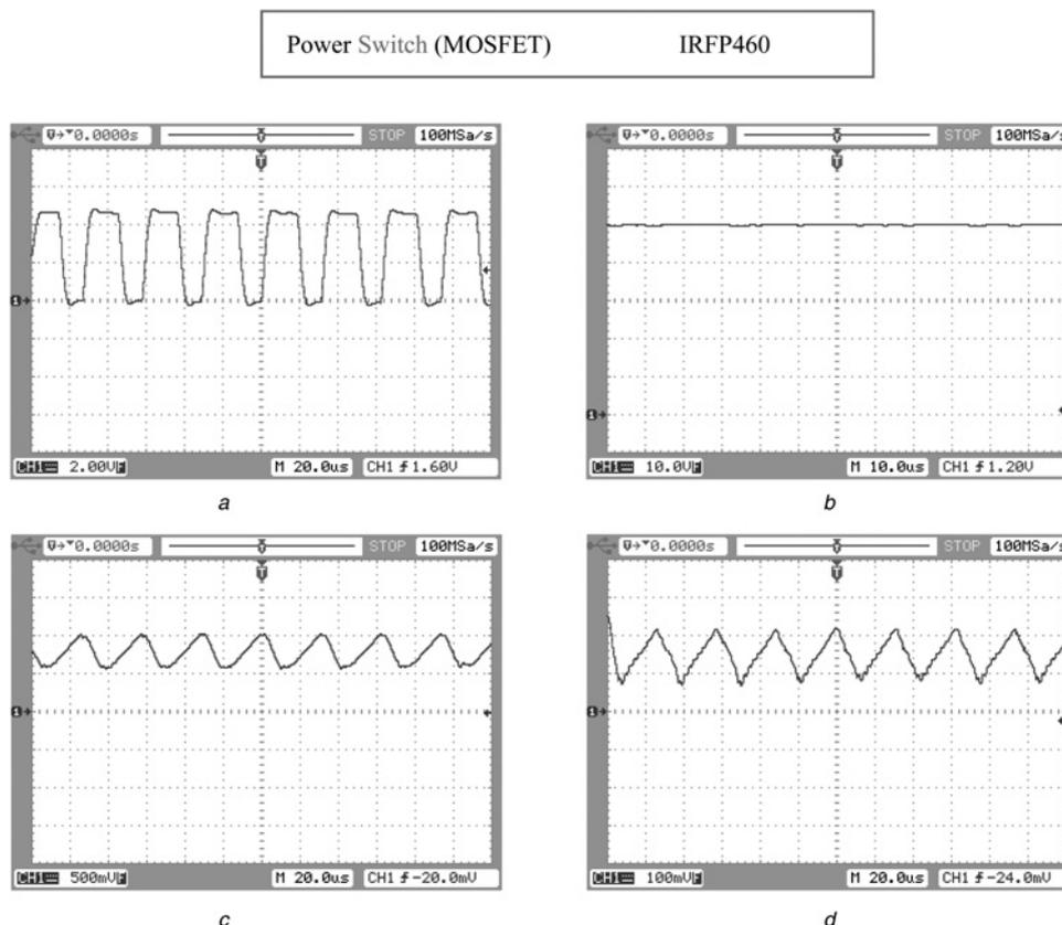
**Fig. 9** Typical waveforms in CCM
