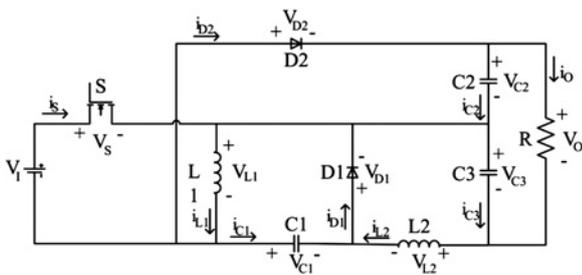
Fig. 1 Circuit configuration of the proposed converter
