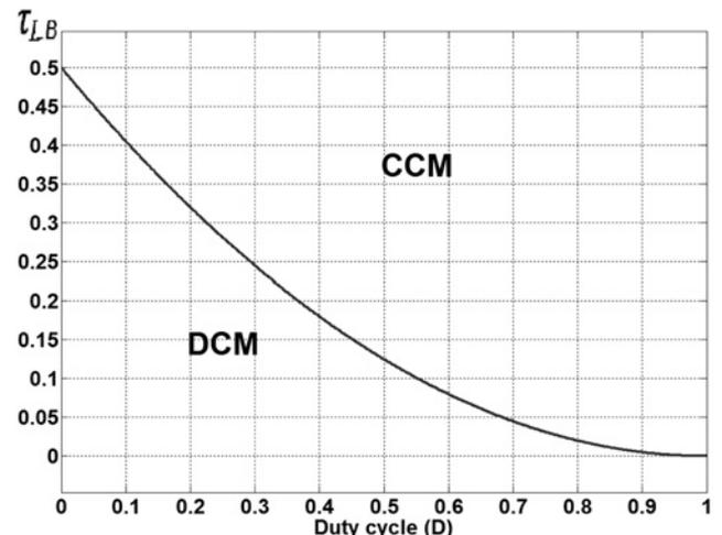
Fig. 5 Boundary condition of the proposed converter
