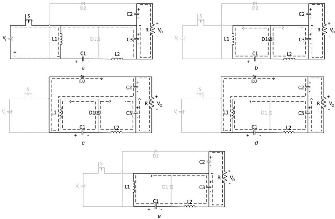
**Fig. 3** Current flow path of the proposed converter in CCM operation
