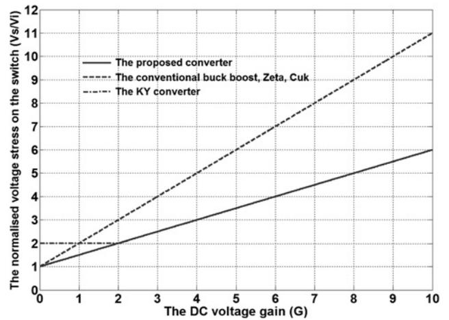
Fig. 6 Voltage stress comparison of the different converters
