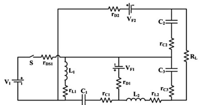
Fig. 7 Equivalent circuit of proposed converter with parasitic resistances and diode forward conducting voltage
