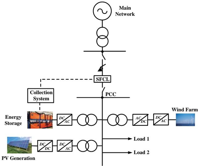
Fig. 2. Schematic diagram of a typical micro-grid integrated with the SFCL.
