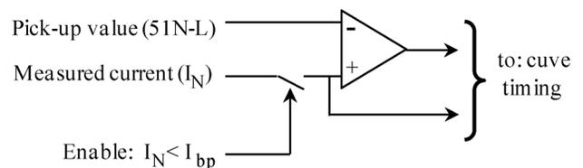
Fig. 6. Example of a way for programming the 51N-L function of Fig. 5 by applying the available options in a commercial relay [32].
