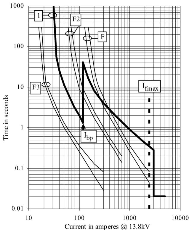
Fig. 10. Case of Fig. 3, considering three different downstream fuses and the aforementioned nontraditional curves for the 51N function.
