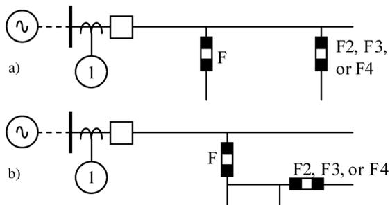
Fig. 9. Examples of configurations with downstream fuses: (a) F2, F3, or F4 are in a different branch than F. (b) F2, F3, or F4 are downstream of F.
