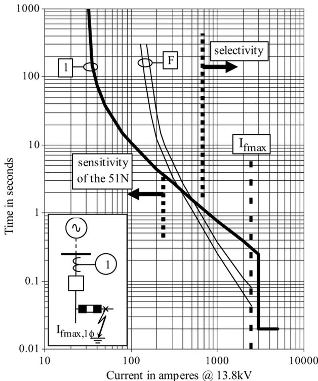
Fig. 1. Traditional coordination of the ground overcurrent function with downstream fuses. There are crossings between curves, but this is the best traditional solution for this case.
