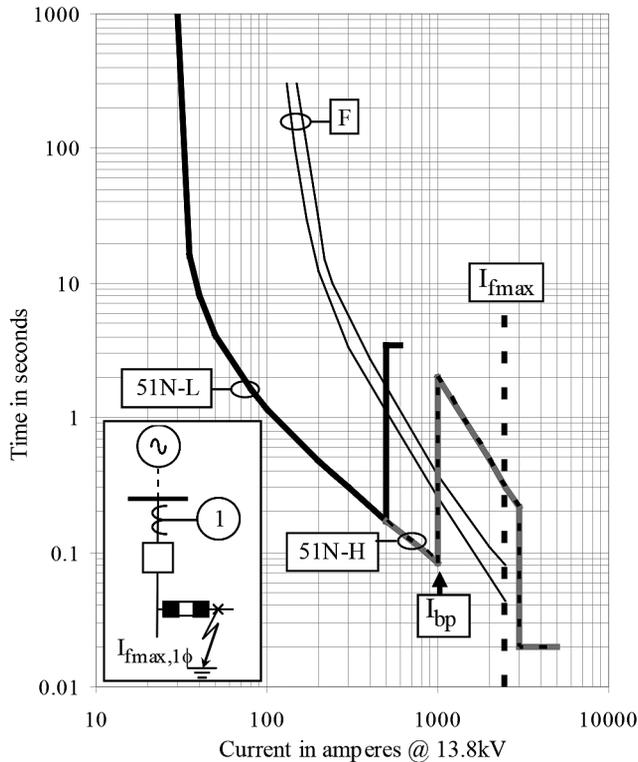
Fig. 7. Case of Fig. 4, implemented by applying curve shapes created by the user (limits in curve shapes for  $M \geq 20$  are considered).
