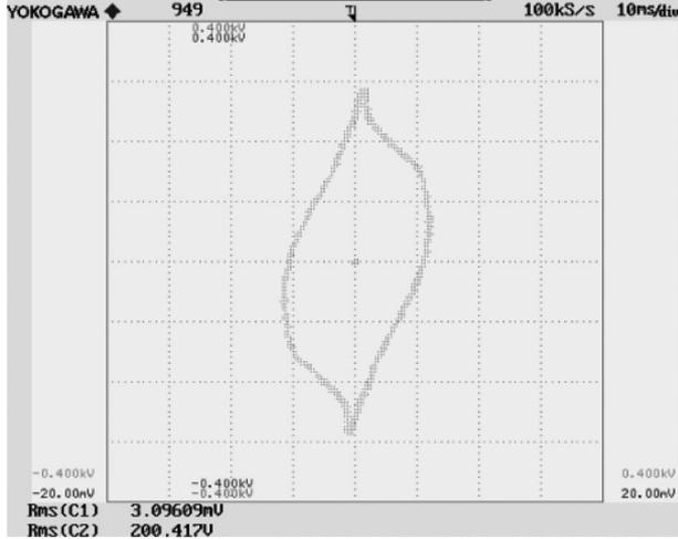
Fig. 9. Lissajous pattern of input voltage versus input current (measured with current probe of 100 mV = 1 A) showing core loss.
