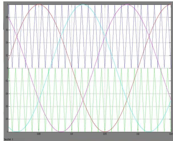
Fig 4. Control Pulse Generation in Three Level SPWM
