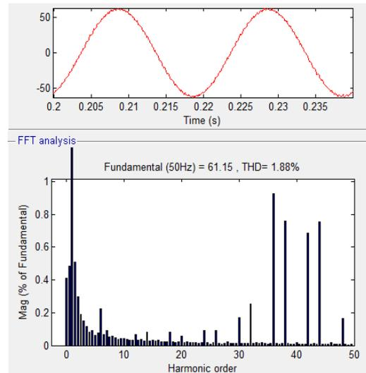
Fig 8. Harmonic spectrum Line current of 3-level inverter for R= 15, L=24.2 mH
