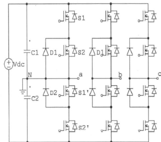
Fig. 1 Diode Clamped Three Level Inverter
