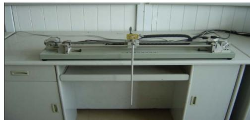
Fig.1 The inverted pendulum used in control laboratories
