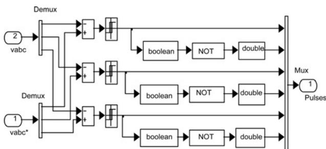
Figure 5 SIMULINK diagram showing the hysteresis voltage controller
