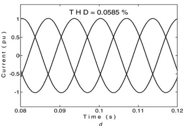
**Figure 12** Steady-state harmonic compensation (linear load)
