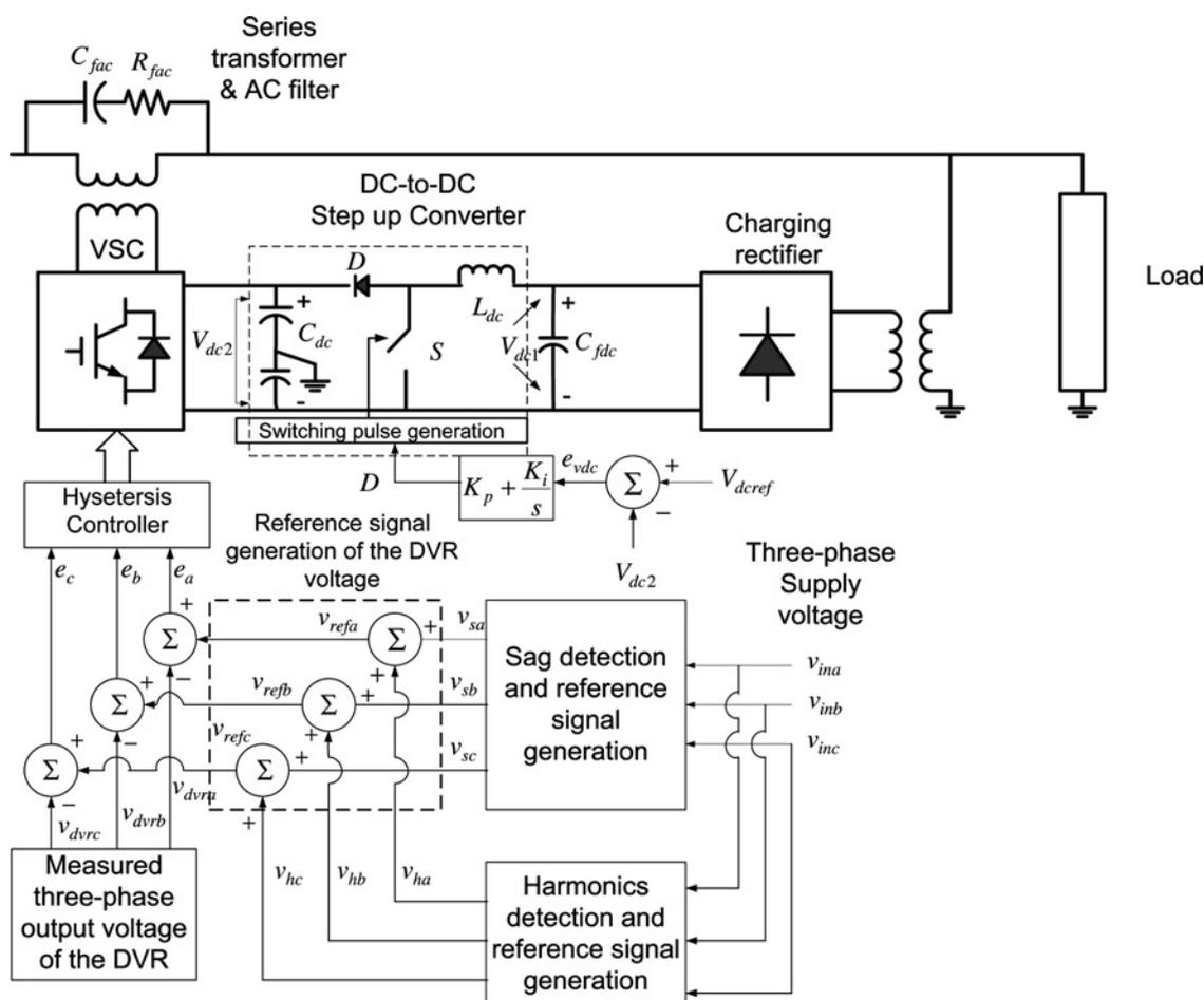
Figure 1 Schematic diagram of the proposed DVR
