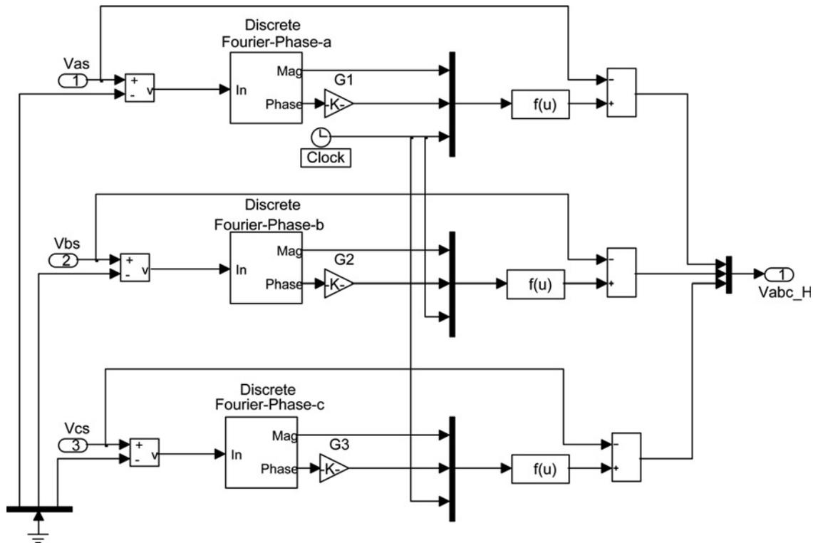
Figure 4 SIMULINK diagram of the harmonics detection scheme
