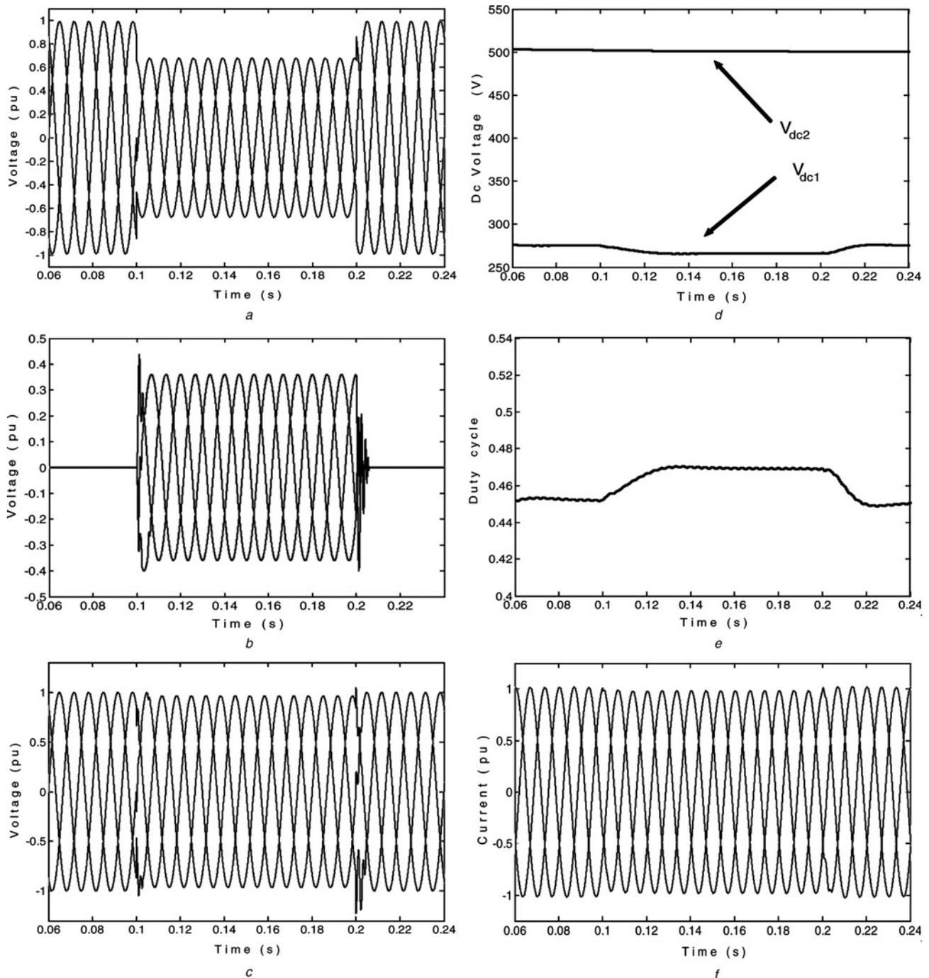
**Figure 10** System response because of three-phase 60% voltage sag with  $+28^\circ$  phase jump (linear load)
