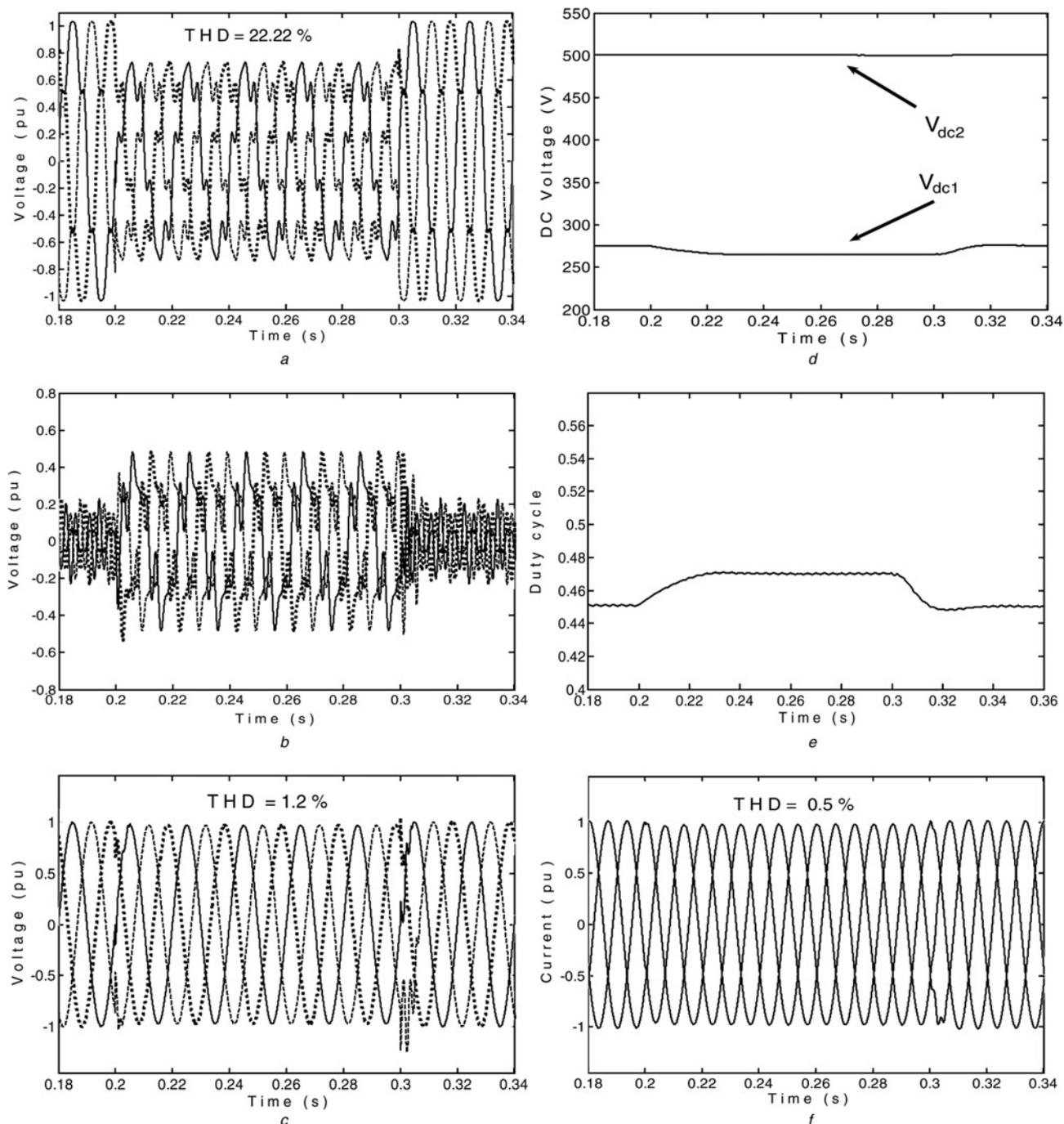
**Figure 14** Three-phase 60% voltage sag with +28° phase jump (linear load) and harmonic compensation
