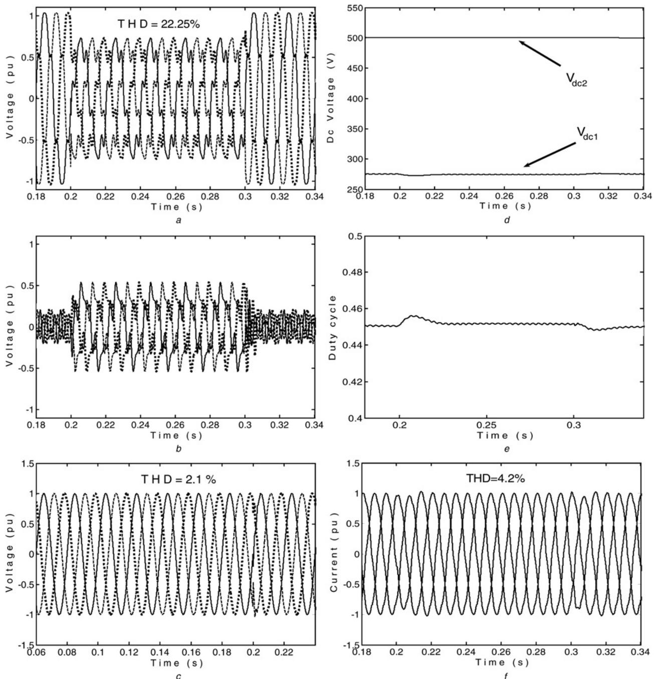
**Figure 15** Three-phase 60% voltage sag with +28° phase jump (non-linear load) and harmonic compensation
