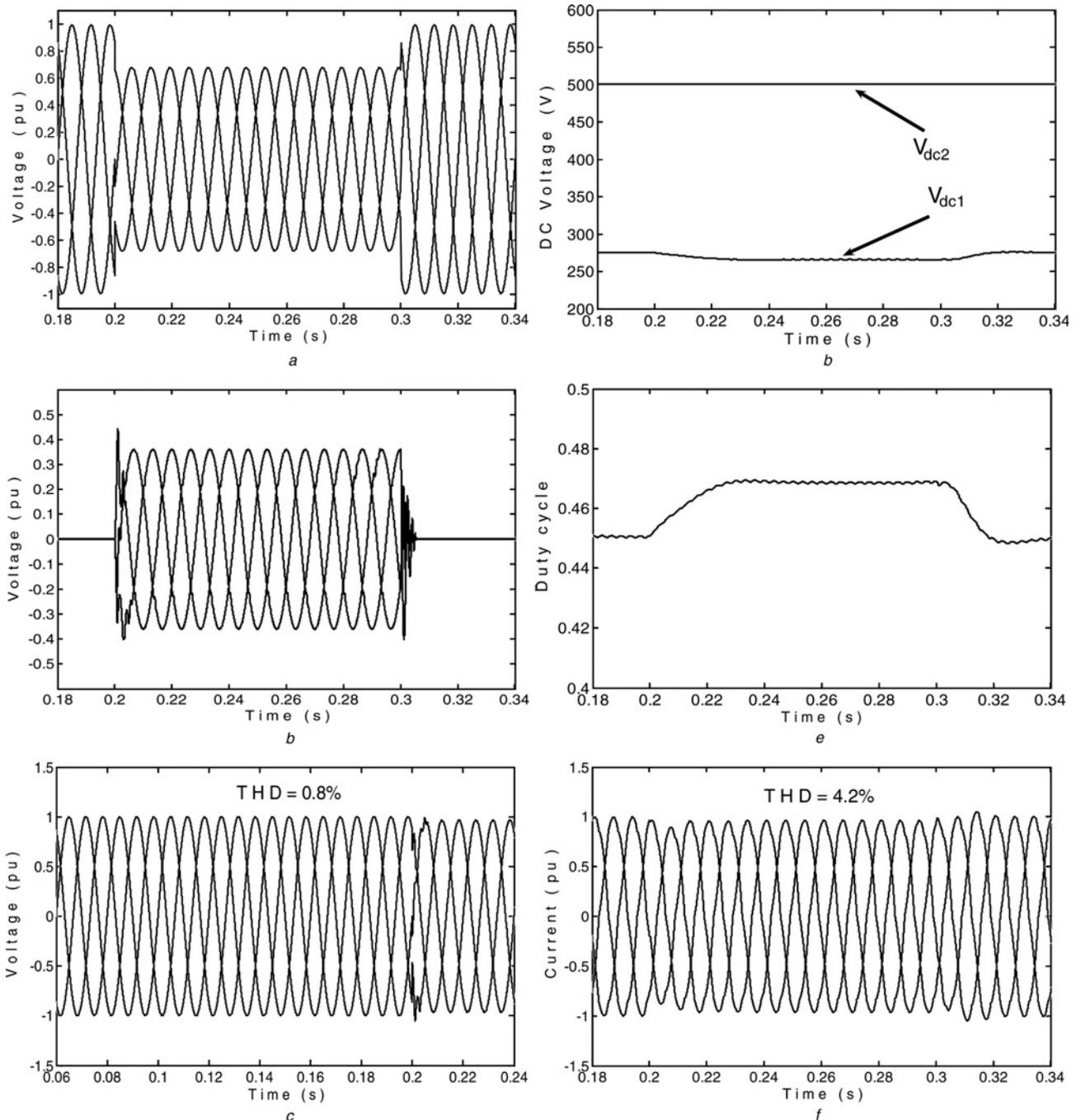
**Figure 11** System response because of three-phase 60% voltage sag with +28° phase jump (non-linear load)
