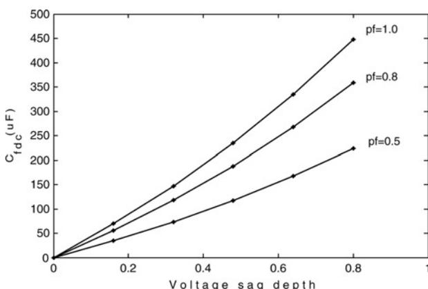
**Figure 7** Relation between dc capacitor  $C_{f_{dc}}$  and voltage sag depth ( $D_{sag}$ )
