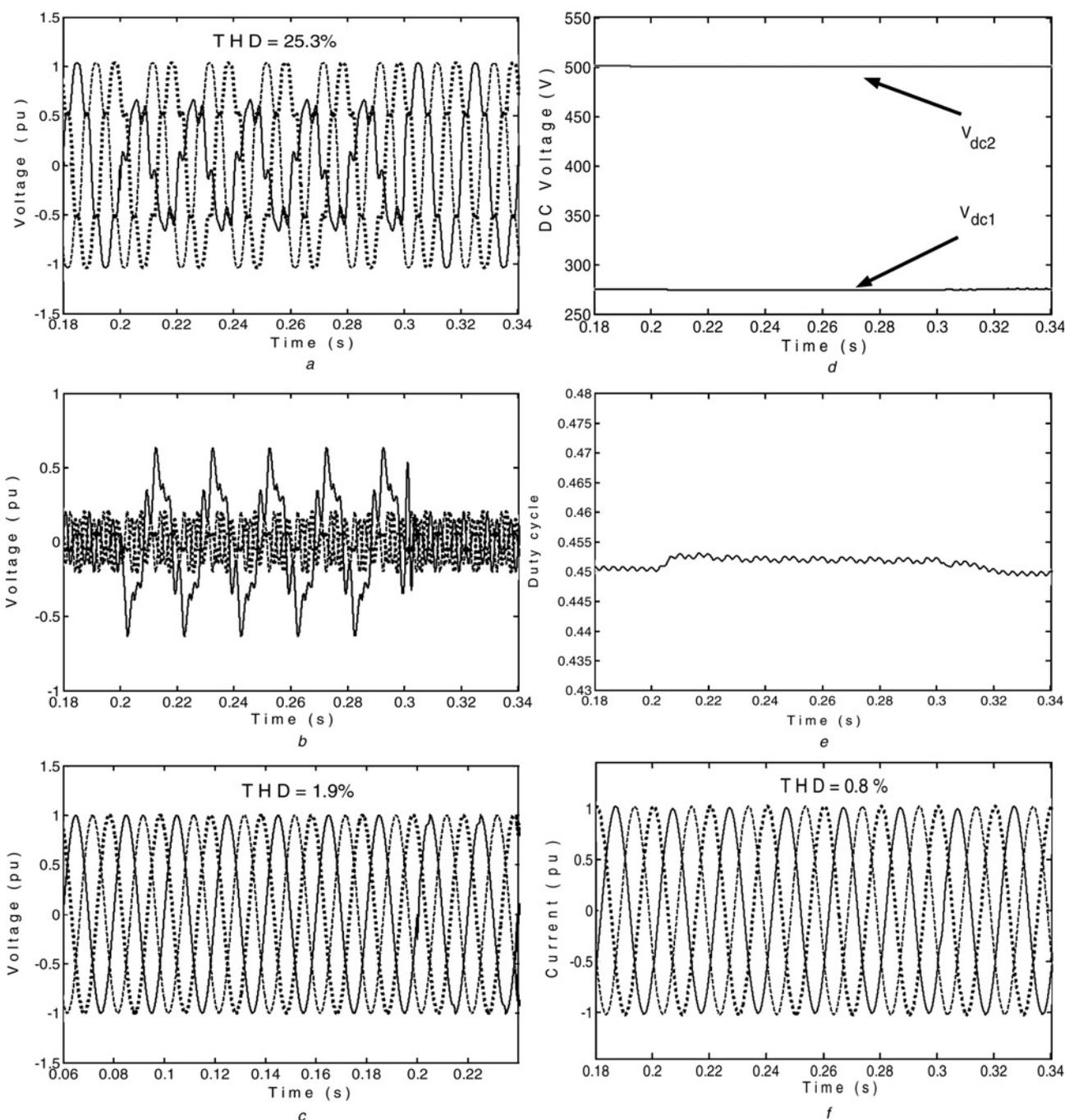
**Figure 16** Single-phase 50% voltage sag with +28° phase jump (linear load) and harmonic compensation
