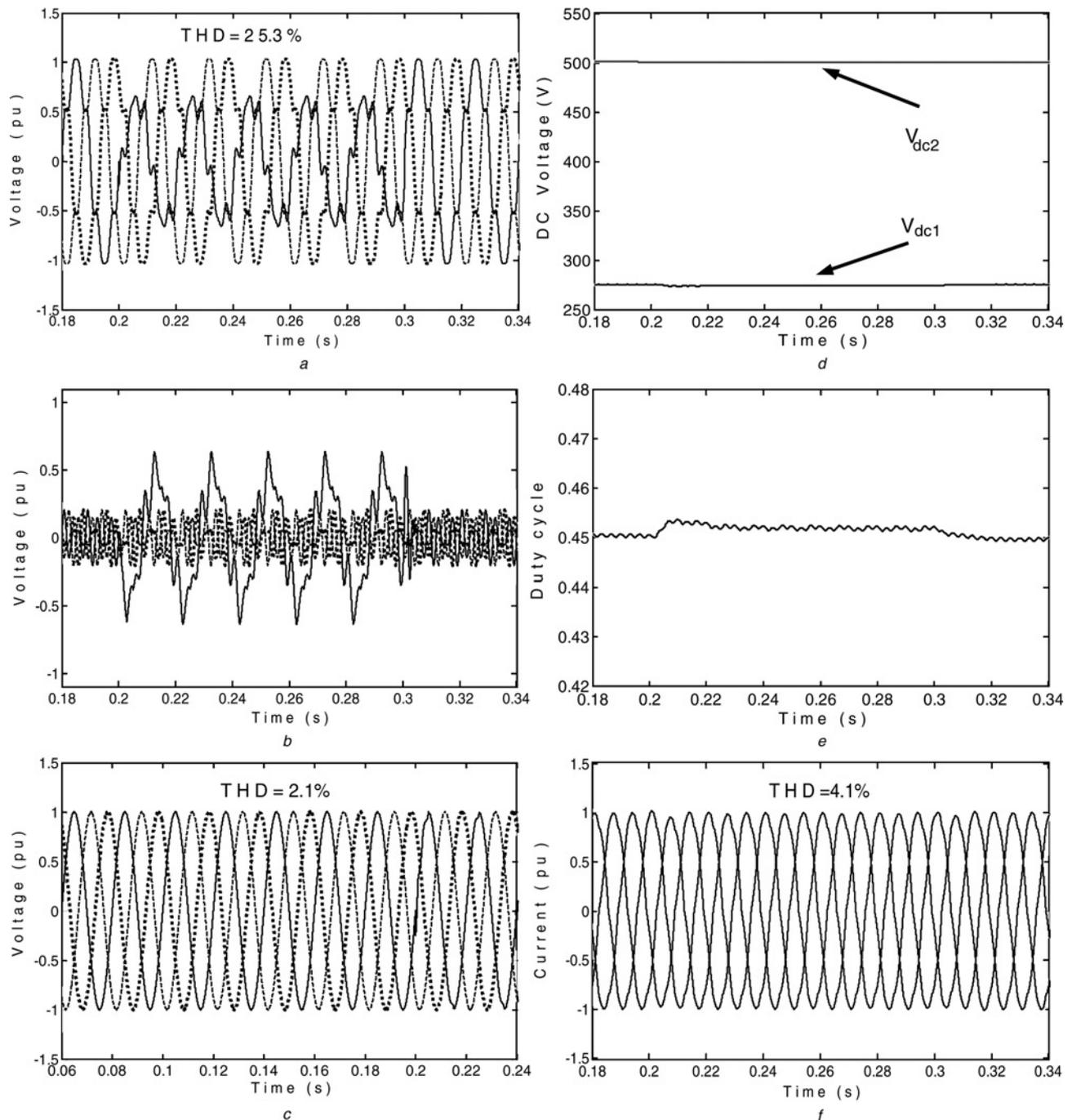
**Figure 17** Single-phase 50% voltage sag with +28° phase jump (non-linear load) and harmonic compensation
