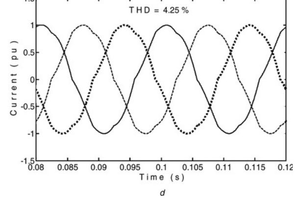
**Figure 13** Steady-state harmonic compensation (non-linear load)
