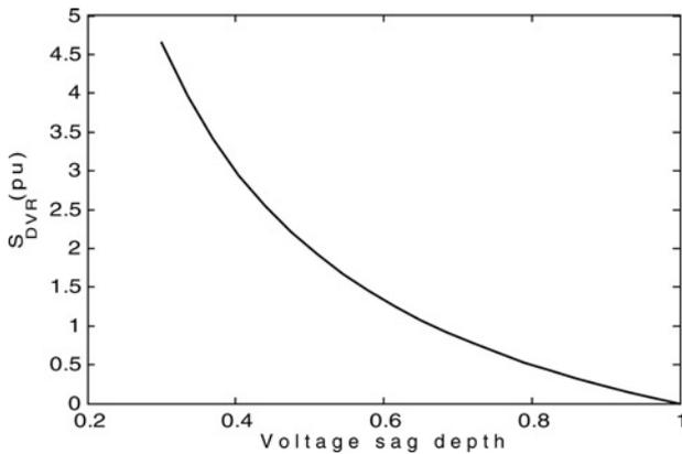
**Figure 6** Overall power rating of the DVR converters as function of the voltage sag depth ( $D_{sag}$ )
