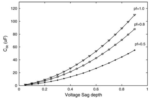
Figure 9 Relation between capacitor  $C_{dc}$  and voltage sag depth ( $D_{sag}$ )
