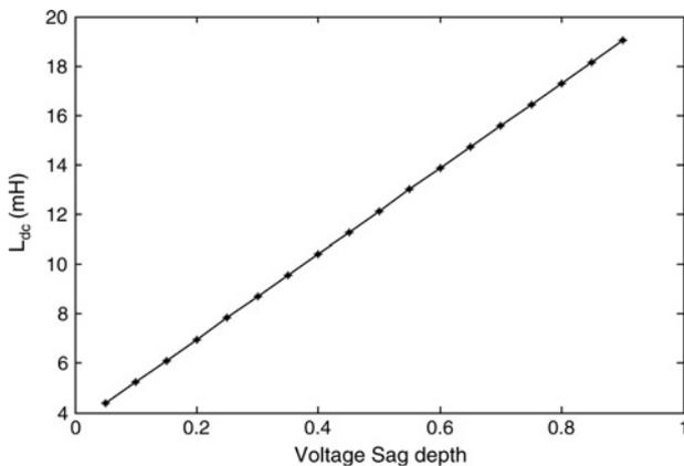
Figure 8 Relation between inductor  $L_{dc}$  and voltage sag depth ( $D_{sag}$ )
