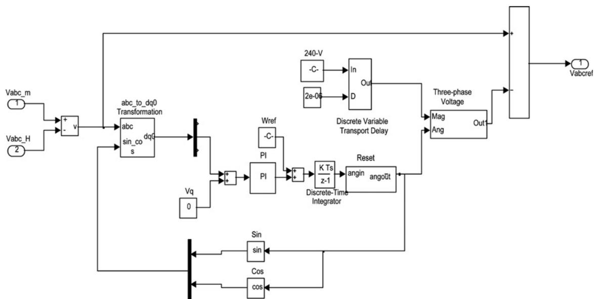
**Figure 3** SIMULINK diagram of the voltage sag detection
