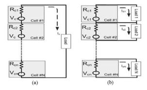
Fig. 5. Modular fuel cell simplified equivalent circuit.
