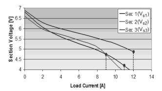
Fig. 7. V-I characteristics of the proposed modular fuel cell stack with three sections
