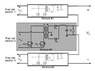
Fig. 9. Proposed modular dc-dc converter.
