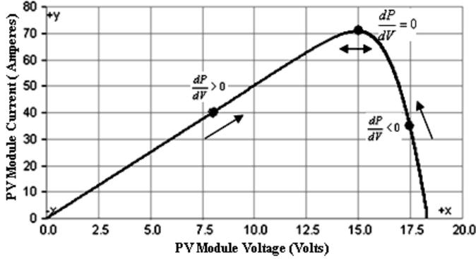
Fig.7. P-V characteristics of the module.
