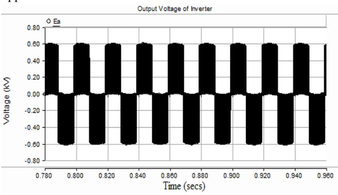
Fig.11 Output voltage of modular multilevel converter.
