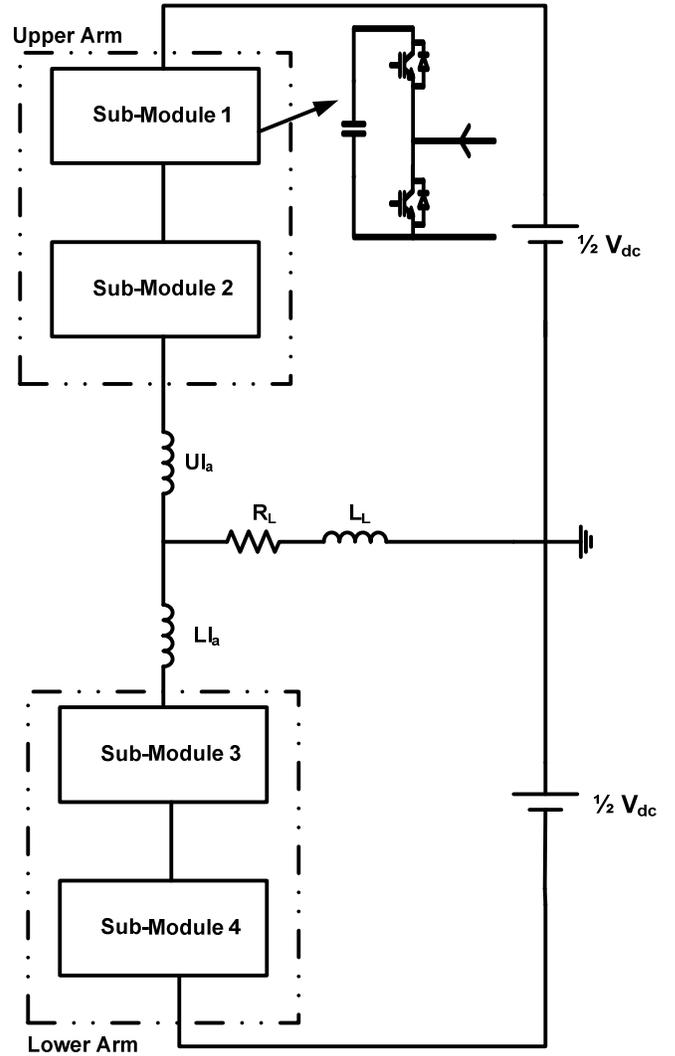
Fig. 5. Single phase of three level modular multilevel converter.
