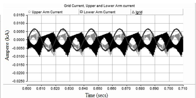
Fig.15 Grid current, lower arm current and upper arm current.
