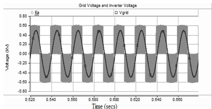
Fig.14 Grid voltage and MMC output voltage.
