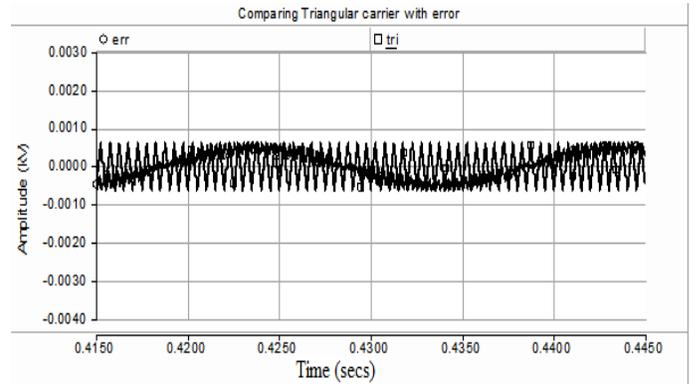
Fig.13 Triangular carrier comparison with the error signal.
