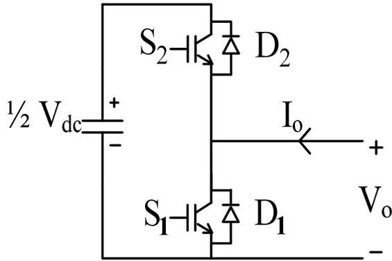
Fig. 4. Structure of one sub-module.
