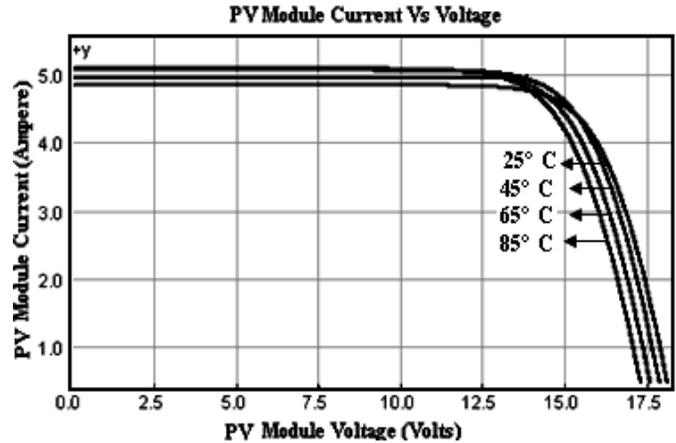
Fig. 3. Current versus voltage at constant solar radiation  $G = 1000 \text{ W/m}^2$ .
