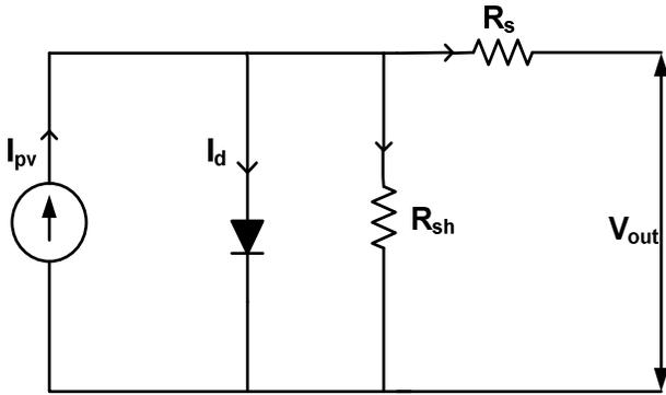
Fig.1. Electrical equivalent circuit of PV cell.
