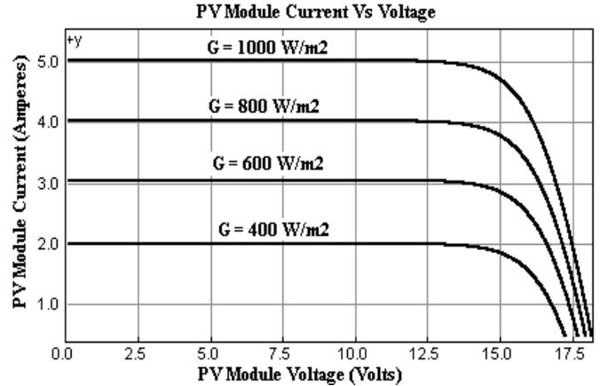
Fig.2. Current versus voltage at constant cell temperature  $T = 25^\circ\text{C}$ .
