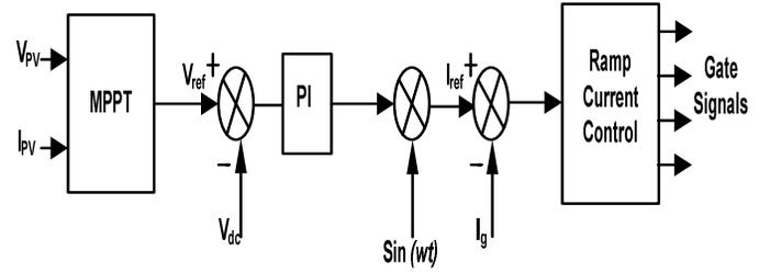
Fig. 8. Block diagram of outer and inner control loop.
