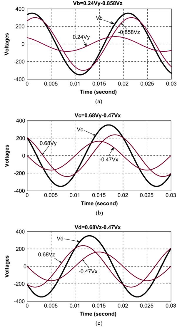
Fig. 5(a)–(c). (a) Input  $V_y$  and  $V_z$  phases and output  $V_b$  phase voltage waveforms. (b) Input  $V_y$  and  $V_x$  phases and output  $V_c$  phase voltage waveforms. (c) Input  $V_z$  and  $V_x$  phases and output  $V_d$  phase voltage waveforms.
