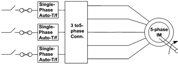
Fig. 7. Circuit diagram for a direct-online start of the five-phase motor.
