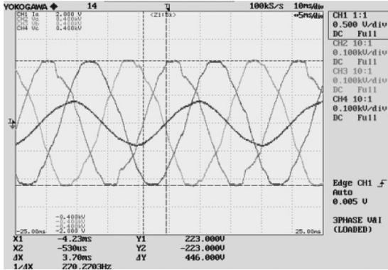
Fig. 8. Input side (three-phase) voltages and current waveform.
