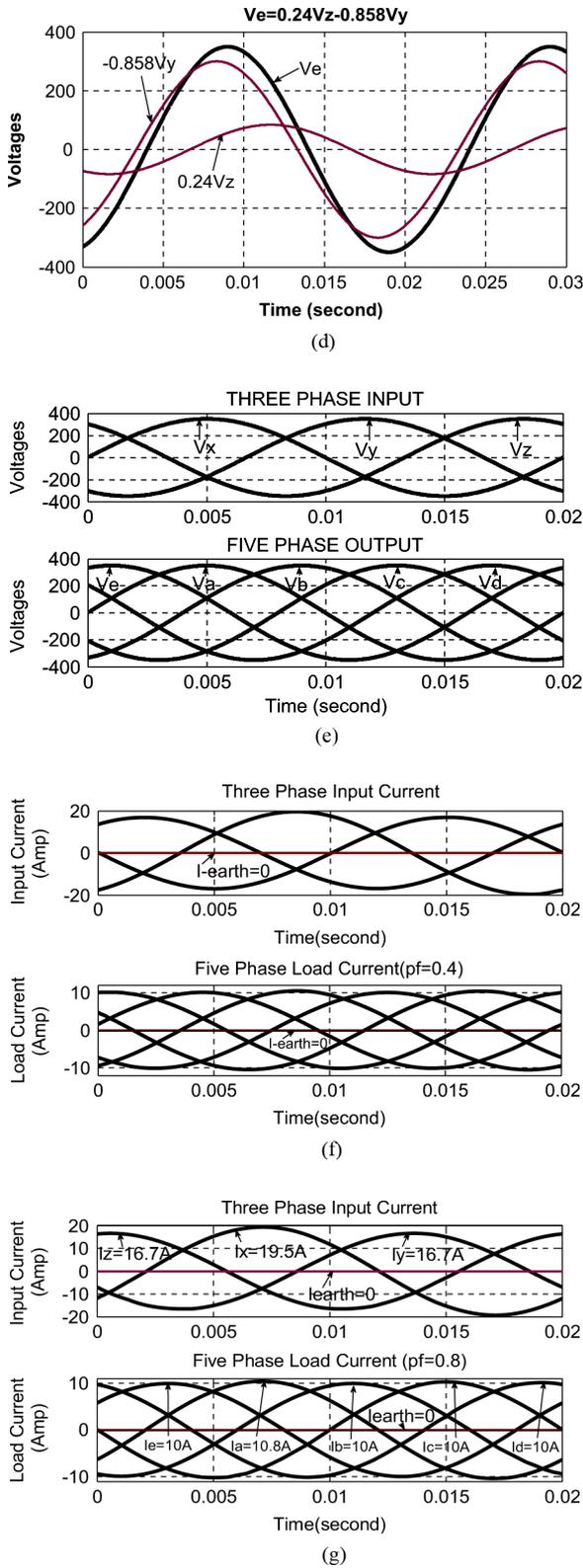
Fig. 5(d)–(g). (d) Input  $V_z$  and  $V_y$  phases and output  $V_e$  phase voltage waveforms. (e) Input three-phase and output five-phase voltage waveforms. (f) Input three-phase and output five-phase load current waveforms at  $PF = 0.4$ . (g) Input three-phase and output five-phase load current waveforms at  $PF = 0.8$ .
