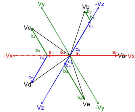
Fig. 3. Phasor diagram of the proposed transformer connection (star-star).
