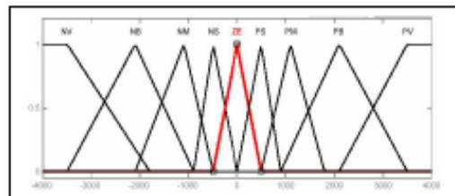
Fig. 5 Membership function for desired actuator force
