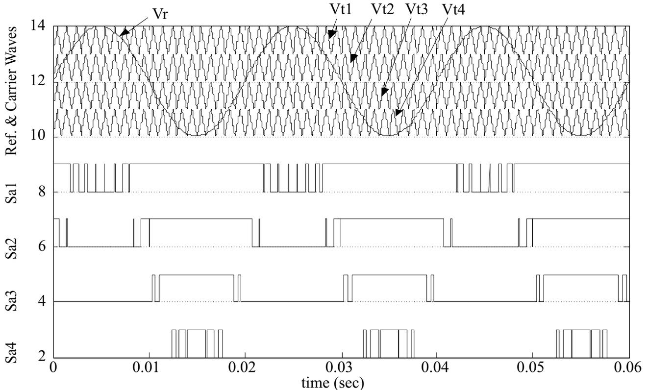
**Figure 8: Pulse generation for five-level inverter (for switches Sa<sub>1</sub>, Sa<sub>2</sub>, Sa<sub>3</sub> and Sa<sub>4</sub>).**
