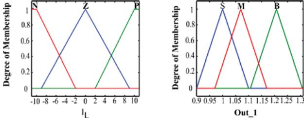
Fig. 6: Membership functions for current fuzzy-logic controller.
