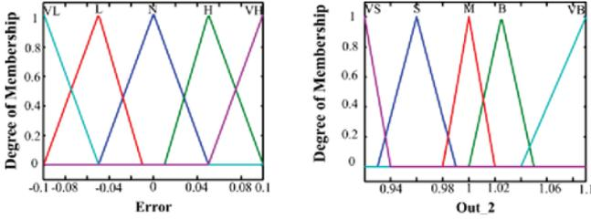
Fig. 7: Membership functions for voltage fuzzy-logic controller.
