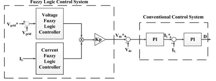
Fig. 5: Block diagram of the proposed control scheme
