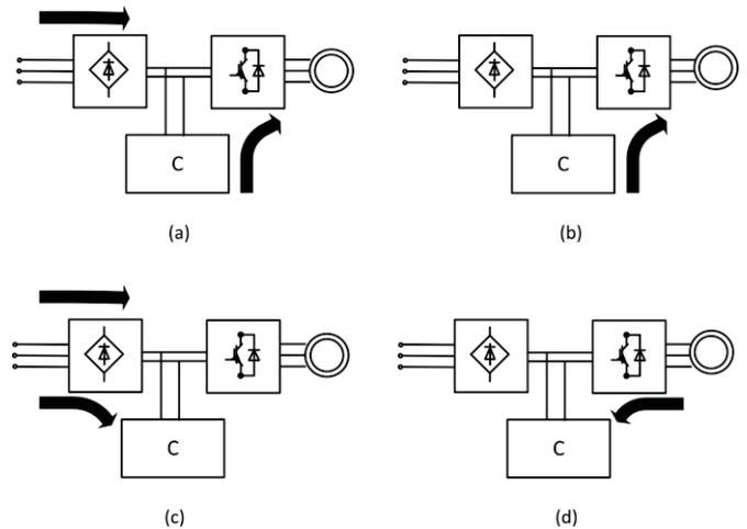
Fig. 3: Energy flow in a motor drive system, with supercapacitors as energy storage device: (a) both grid and supercapacitors supply energy to the motor, (b) motor is supplied only from the energy stored at the supercapacitors, (c) grid supply energy to the motor and for charging the supercapacitors and (d) supercapacitors are charged by the braking energy of the electric machine.
