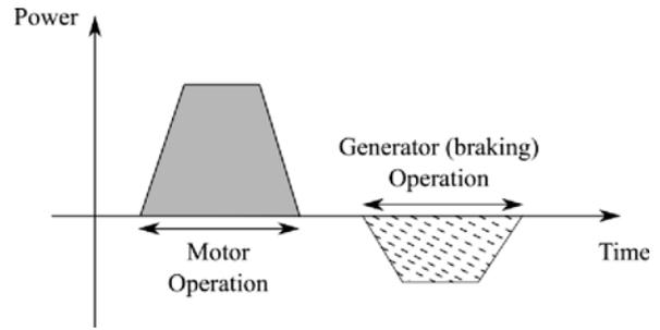
Fig. 2: Typical diagram of energy flow in an elevator operation cycle.
