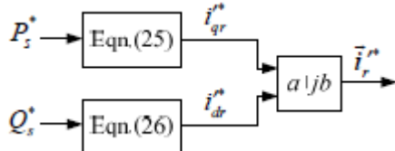
Fig 5. Reference calculation block for rotor-side level 1.
