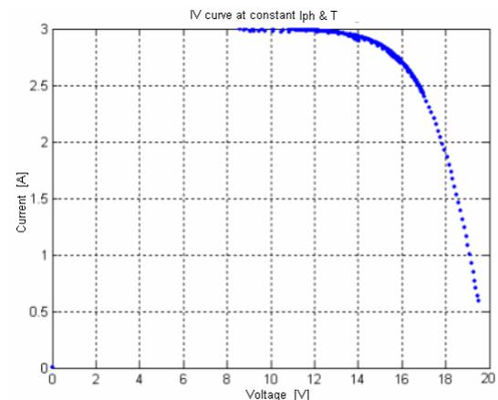
Fig. 12:  $I \times V$  characteristic curve of the solar panel.
