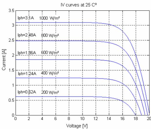
Fig. 4:  $I \times V$  characteristic of solar panel with 36 cells.
