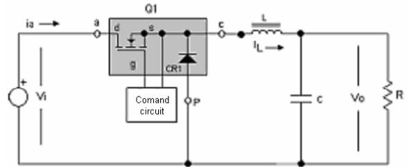
Fig. 6: Simplified diagram of a converter buck.
