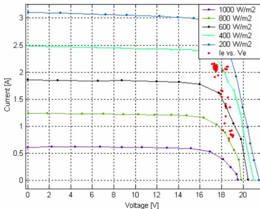
Fig. 17: Operation points of the solar panel with MPPT control, considering a resistive load equal to  $5\Omega$ .
