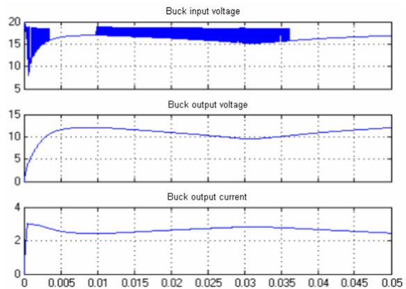
Fig. 11: Output waveforms obtained by simulation of the chopper with resistive load.
