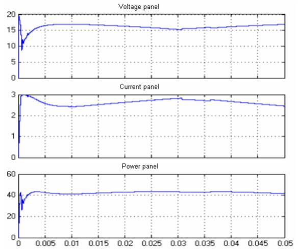
Fig. 10: Output signals of the solar panel with resistive load variable.
