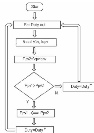
Fig. 7: Flow chart of the P&O control algorithm.
