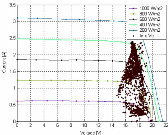
Fig. 18: Operation points of the solar panel with MPPT control, considering as a 12VDC battery charge.
