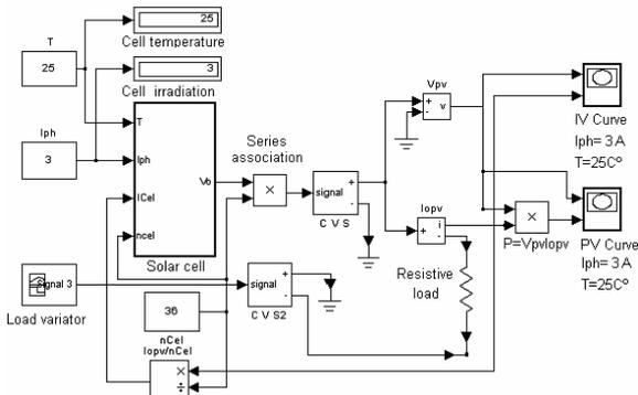
Fig. 3: Diagram for the simulation of the solar panel.
