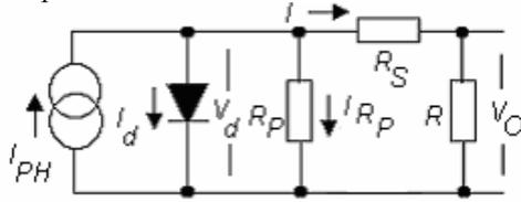
Fig. 1: Circuit equivalent of complete solar cell, considered the internal losses.
