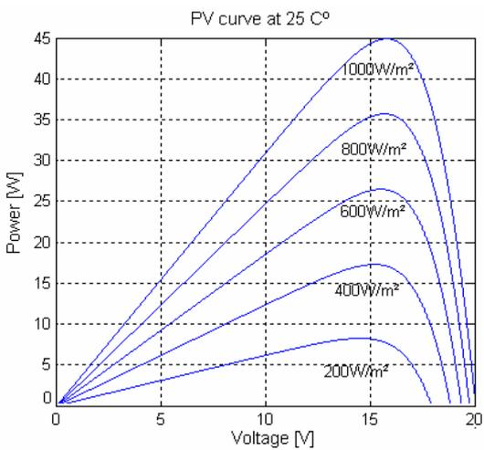
Fig. 5:  $P \times V$  curves of solar panel with 36 cells.
