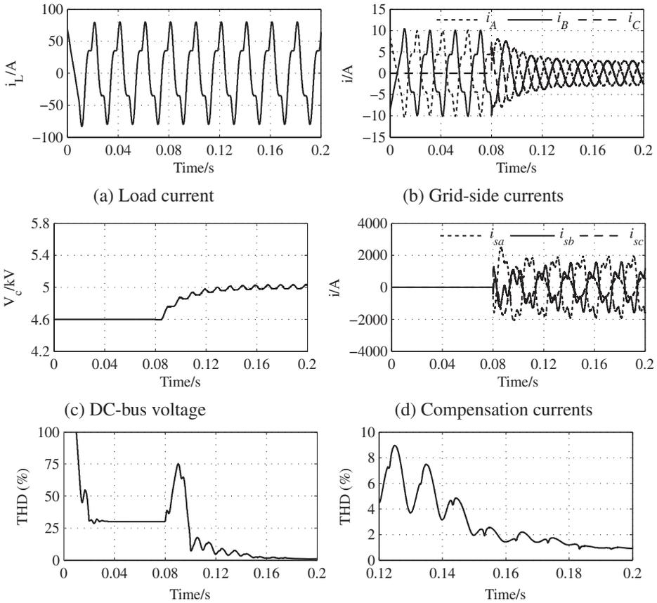
(e) THD of Phase-A grid-side current (f) THD of Phase-A grid-side current (0.12~0.2 s)
