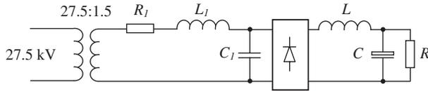
**Figure 9.5** Load model of a high-speed train
