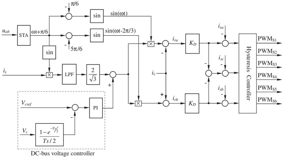
**Figure 9.3** Control strategy to compensate negative-sequence, reactive and harmonic currents
