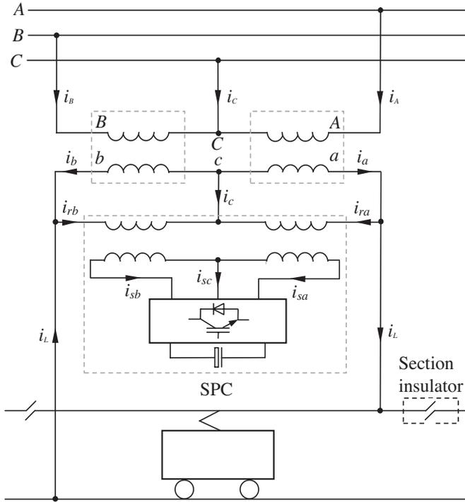
**Figure 9.1** Traction power system with a single feeding wire equipped with a V/V transformer
