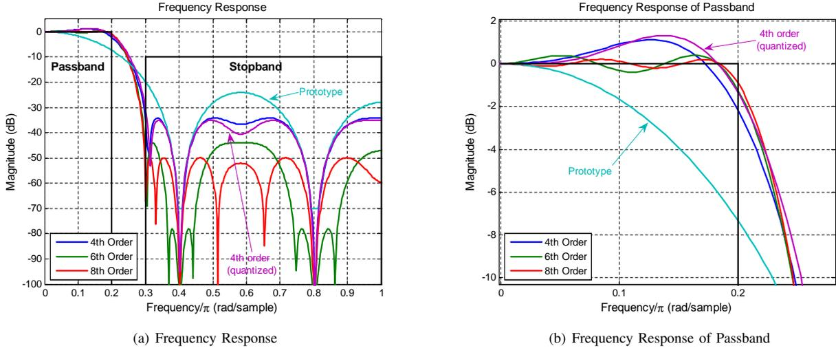
Fig. 4. Frequency Response of 5-fold Decimation Filter whose target output rate is the Nyquist Rate.
