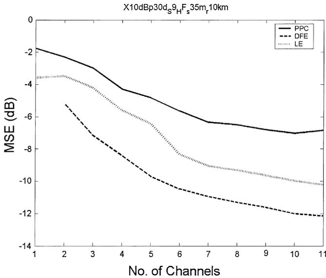
Fig. 13. The mse as a function of the number of receivers for PPC (solid line), LE (dotted line), and DFE (dashed line) for the simulated data.
