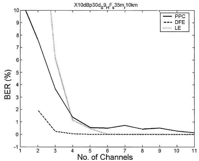
Fig. 15. BER as a function of the number of receivers for PPC (solid line), LE (dotted line), and DFE (dashed line) for the simulated data.
