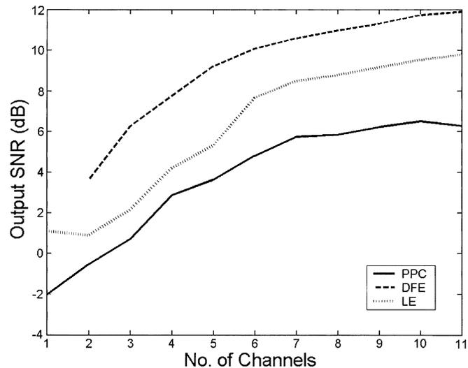
Fig. 14. Output SNR as a function of the number of receivers for PPC (solid line), LE (dotted line), and DFE (dashed line) for the simulated data.
