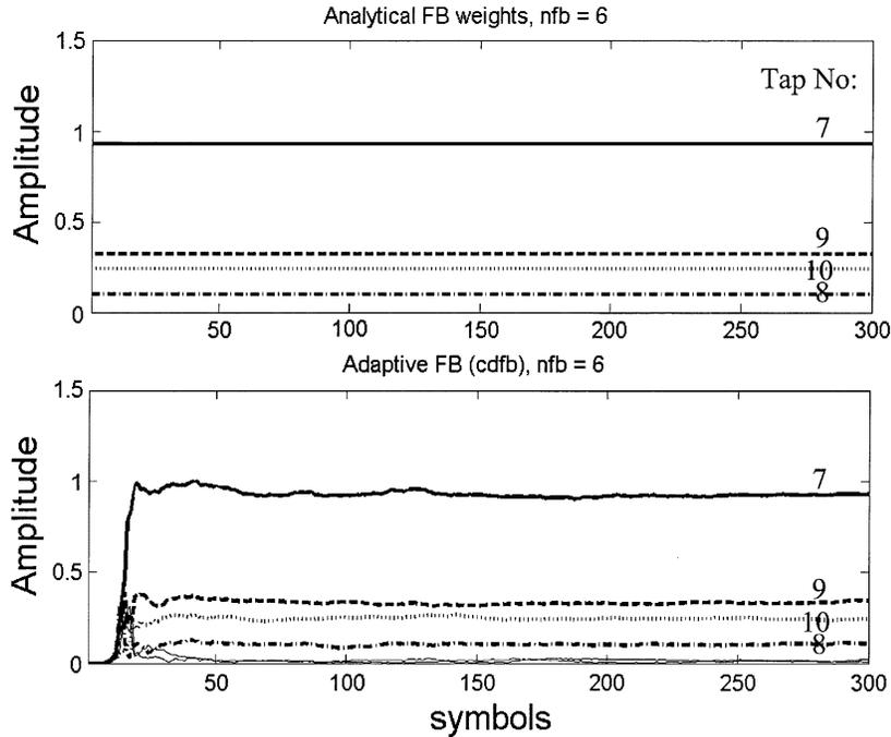
Fig. 6. Evolution of the feedback coefficients as determined by the RLS algorithm (lower figure). The mmse solution for impulse response B of Fig. 4 (upper figure).
