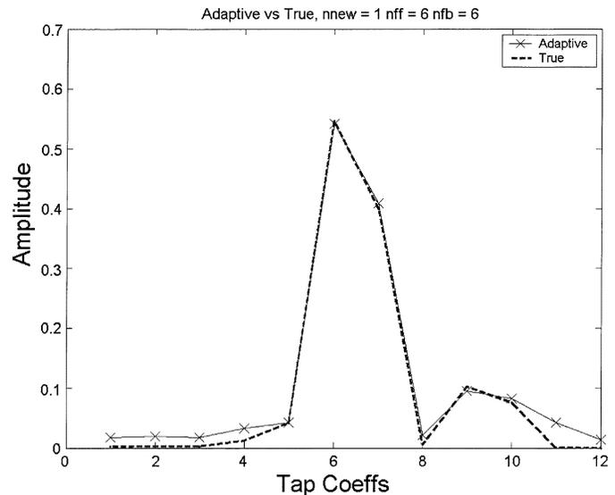
Fig. 8. Comparison of tap coefficients determined by the RLS algorithm ("x" and solid line) and mmse formula (dashed line) for impulse response A of Fig. 4. Feed-forward and feedback are designated by taps 1–6 and 7–12, respectively.
