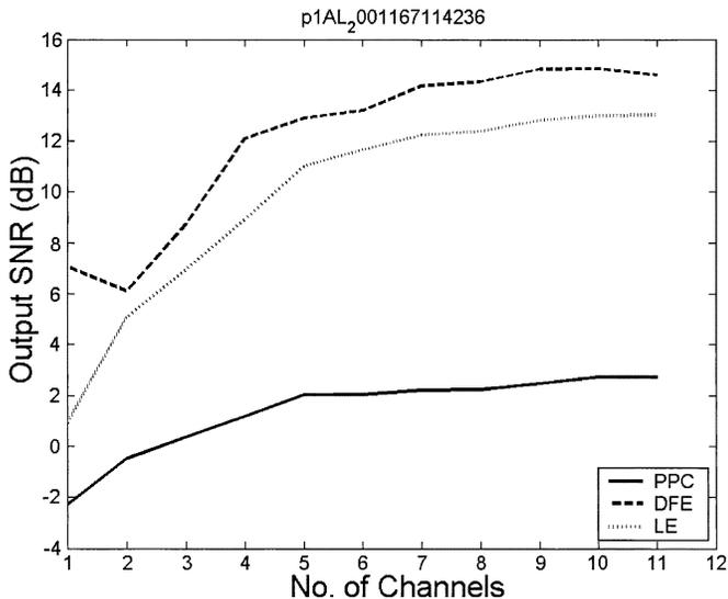
Fig. 20. Output SNR as a function of the number of receivers for (solid line) PPC, (dotted line) LE, and (dashed line) DFE for the ASCOT data.
