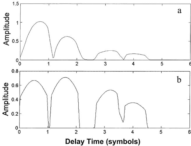
Fig. 4. Band-limited impulse-response functions [impulse responses (a) A and (b) B, respectively] simulating direct, surface, bottom, and surface-bottom bounce arrivals.
