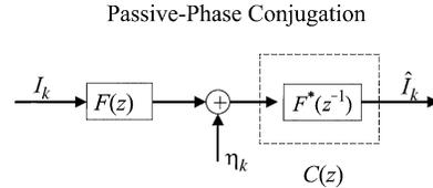
Fig. 3. Block diagram for the PPC equalizer.
