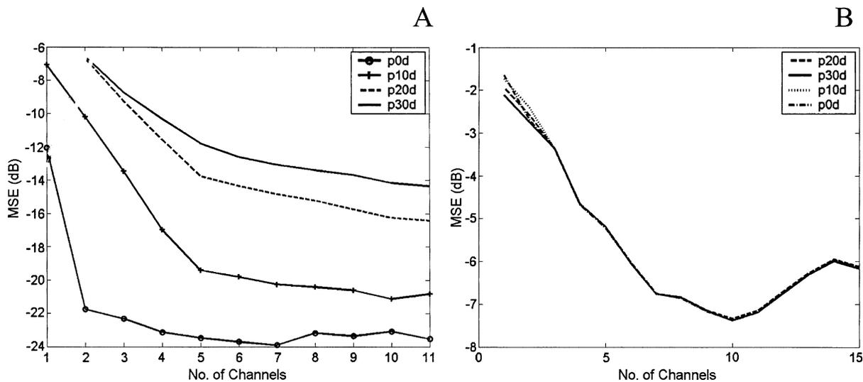
Fig. 16. The mse as a function of the number of receivers: sensitivity to the random-symbol phase with  $\sigma = 0^\circ, 10^\circ, 20^\circ,$  and  $30^\circ$ . (a) DFE and (b) PPC, respectively.
