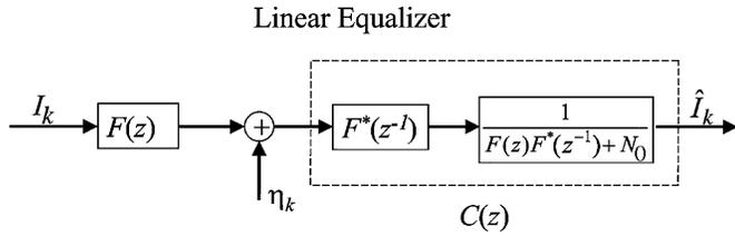
Fig. 1. Block diagram for the LE using the mmse solution.  $F(z)$  is the  $z$  transform of the channel impulse-response function, where  $z = \exp(j\omega t)$ . The equalizer  $C(z)$  reduces to  $1/F(z)$ , the inverse of the impulse-response function, when there is no noise. See [9] for details.
