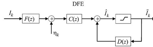
Fig. 2. Block diagram for the DFE.
