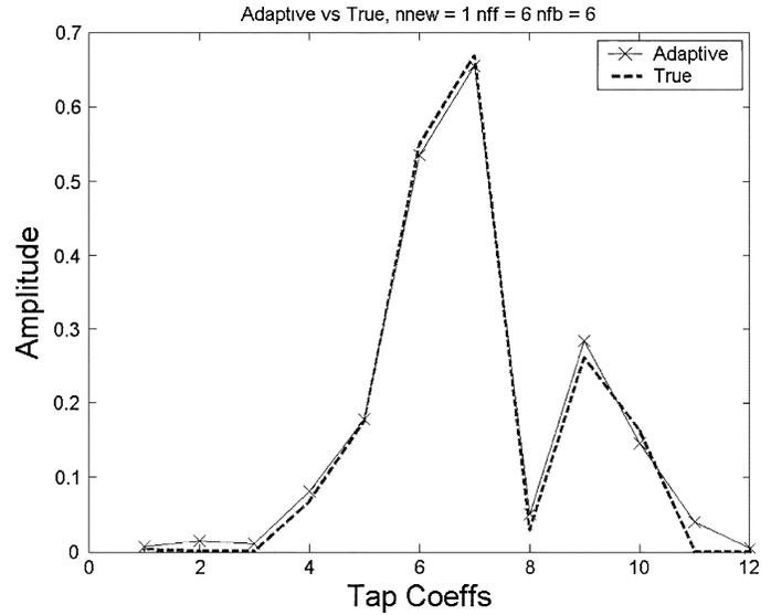
Fig. 5. Comparison of tap coefficients determined by the RLS algorithm (solid line with "x") and mmse formula (dashed line) for impulse response B of Fig. 4. Feed-forward and feedback are designated by taps 1–6 and 7–12, respectively.
