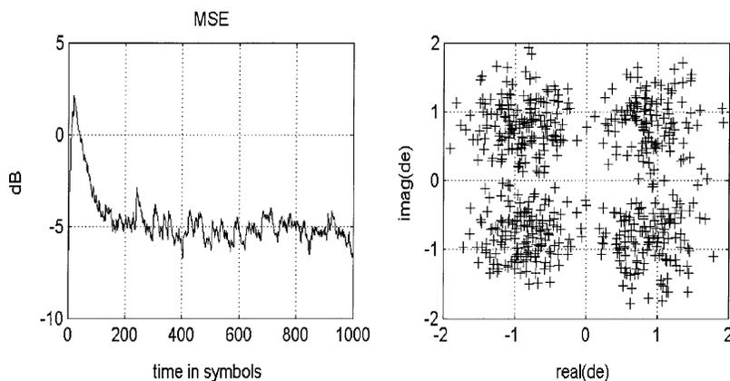
Fig. 10. Symbol mse for impulse response A of Fig. 4 (left) and symbol constellation plot for the estimated symbols,  $d_e$  (right).
