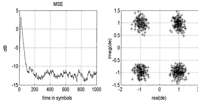
Fig. 7. Symbol mse for impulse response B of Fig. 4 (left). Symbol constellation plot for the estimated symbols,  $d_e$  (right).
