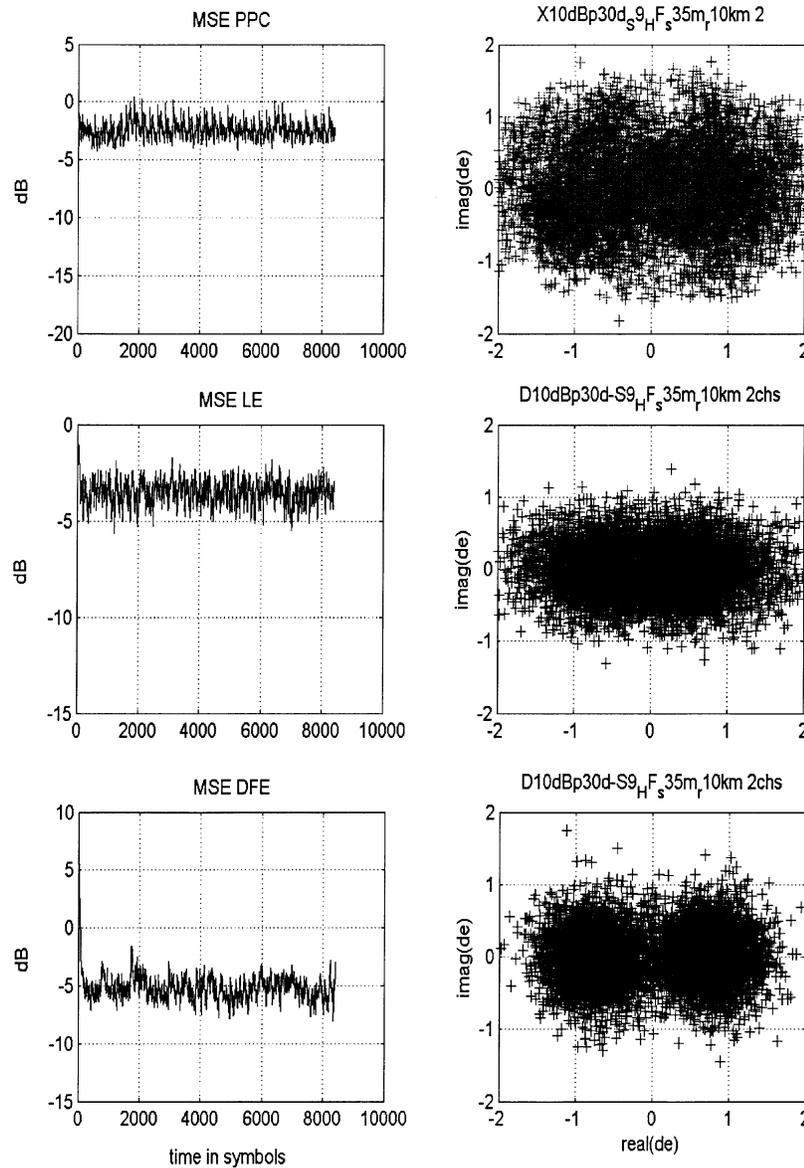
Fig. 11. Analysis of simulated data using the top two receivers. Symbol mse plots are shown on the left and symbol constellation plot for the estimated symbols (de) are shown on the right for the PPC, LE, and DFE processors in descending order.
