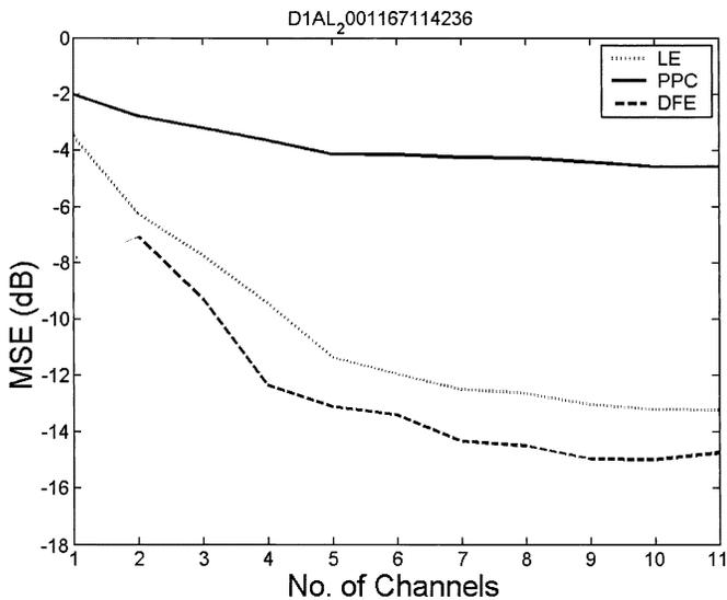
Fig. 19. The mse as a function of the number of receivers for (solid line) PPC, (dotted line) LE, and (dashed line) DFE for the ASCOT data.
