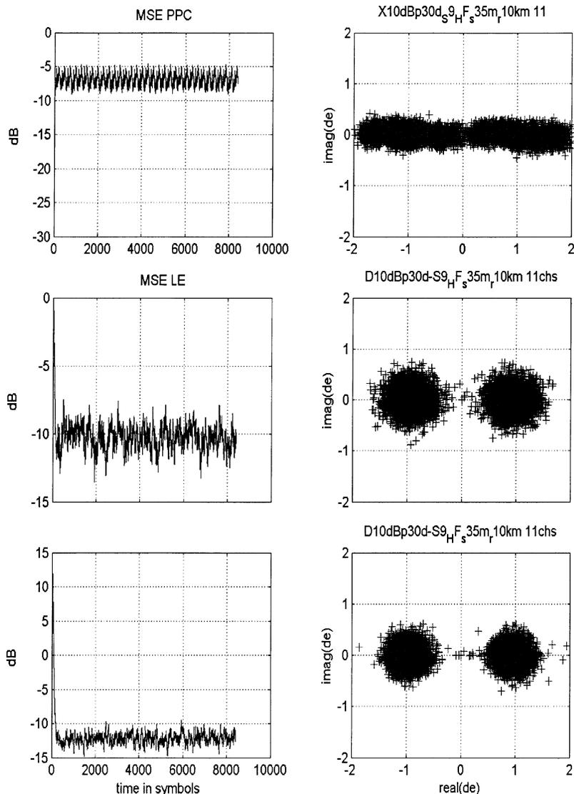
Fig. 12. Analysis of simulated data using 11 receivers. Symbol mse plots (left) and symbol constellation plot for the estimated symbols (de; right) for the PPC, LE, and DFE processors in descending order.
