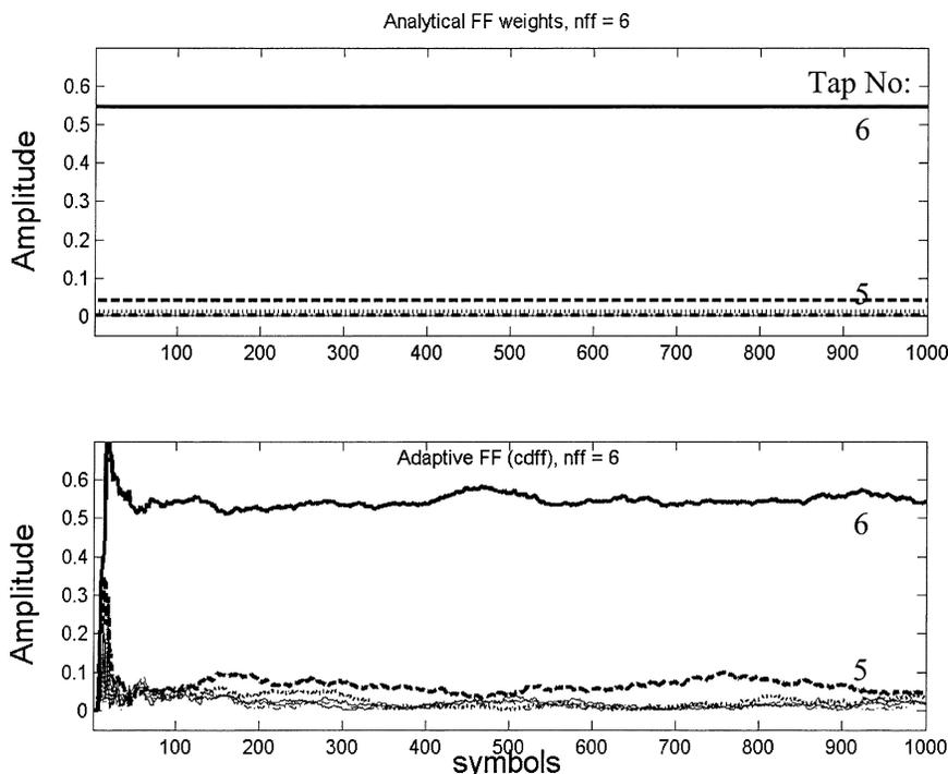
Fig. 9. Evolution of the feedback coefficients as determined by the RLS algorithm (bottom) and mmse solution for impulse response A of Fig. 4 (top).
