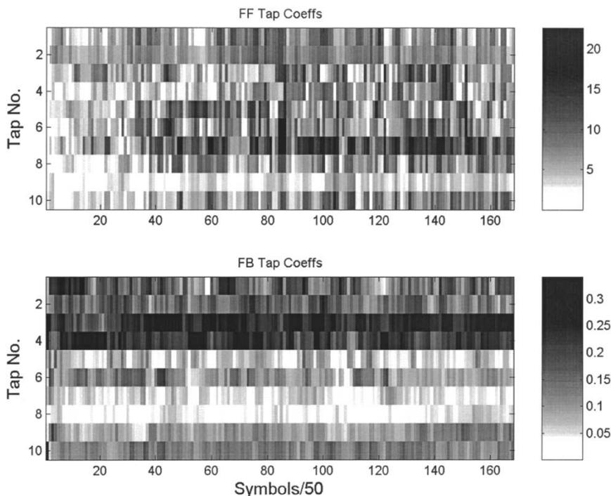
Fig. 22. Time evolution of feed-forward tap coefficients, single channel (top) and first ten feedback tap coefficients (bottom) for the ASCOT data using a four-channel DFE that yields zero bit error.
