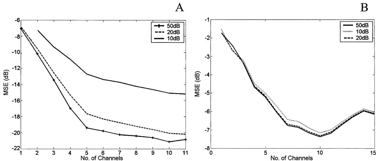
Fig. 17. The mse as a function of the number of receivers: dependence on the SNR for (a) DFE and (b) PPC.
