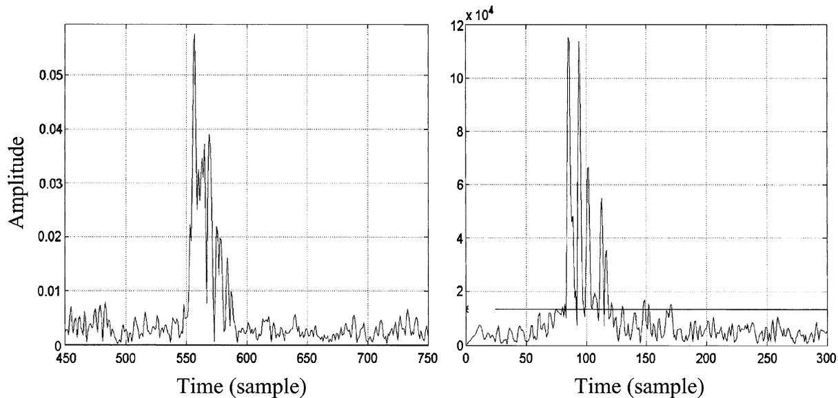
Fig. 18. Comparison of impulse-response functions for (left) simulated data and (right) ASCOT data. Two samples per symbol.
