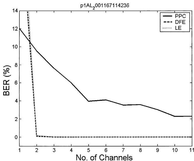
Fig. 21. BER as a function of the number of receivers for (solid line) PPC, (dotted line) LE, and (dashed line) DFE for the ASCOT data.
