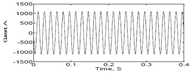
Figure 8. Winding cp current for an internal single phase to ground fault.
