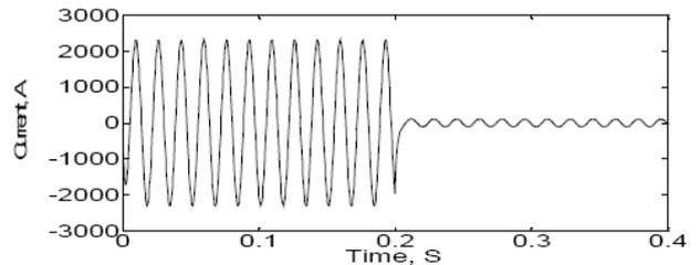
Figure 9. Winding as current for an internal single phase to ground fault.
