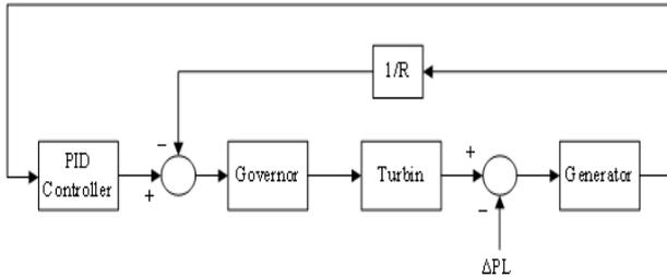
Fig.1. A single area power system with the controllers ( $\Delta PL = 0.01$ )
