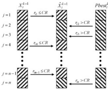
Fig.3. Illustration of crossover operation
