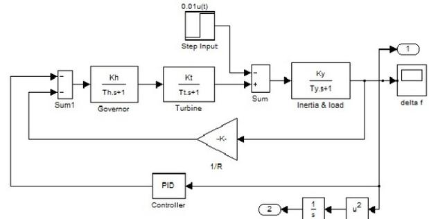
Fig. 4. A single area power system with proposed IPSO-PID controller.
