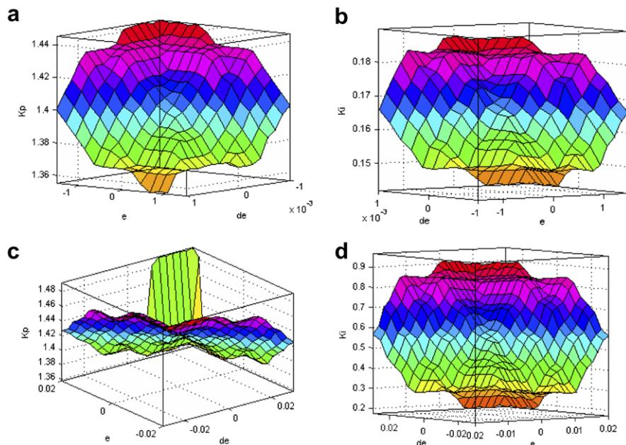
Fig. 9. The variation of  $e$  and  $de$  with respect to  $K_p$  and  $K_i$ : (a–b) surface viewers for two area power system and (c–d) surface viewers for single area power system.
