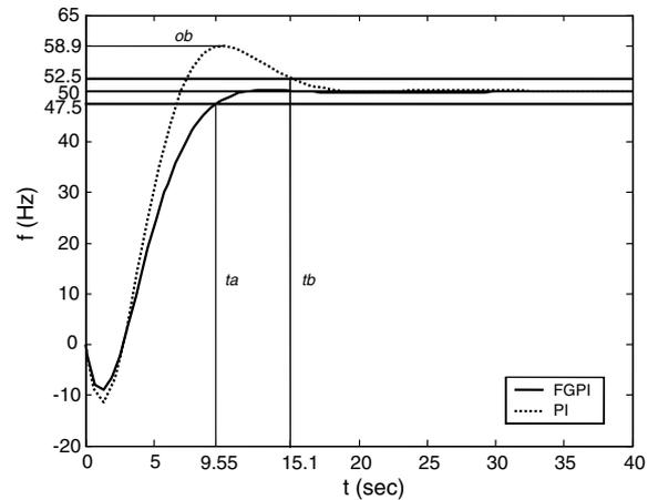
Fig. 5. Output frequencies of the single area power system.
