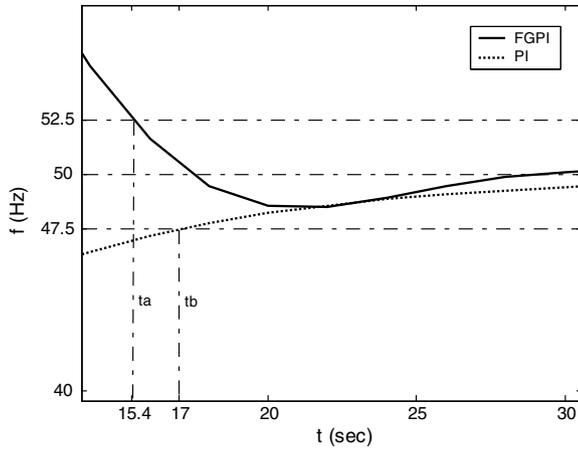
Fig. 7. Output frequencies of the two area power system.
