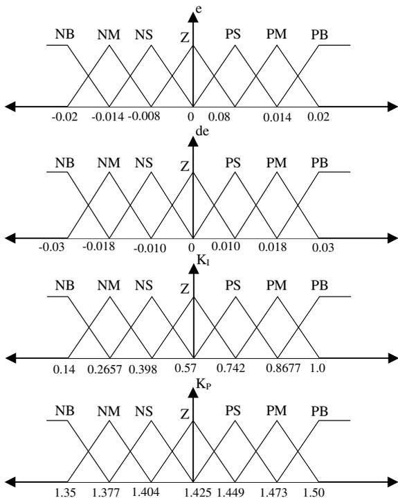
Fig. 4. Membership functions of the FGPI controller.
