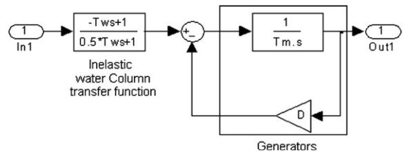
Fig. 1. A single area hydroelectrical power system used in this study.
