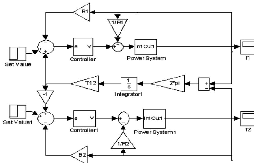
Fig. 2. Two area power system with controllers [10].
