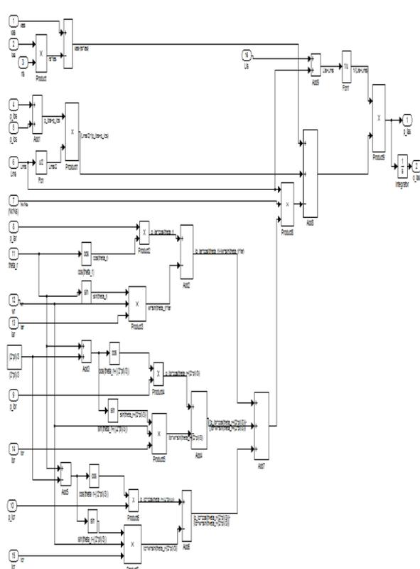
Figure 2 Sub-system of stator current  $i_{as}$
