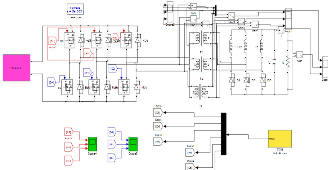
**Fig. 3. Three-phase high frequency isolated DC–DC converter.**
