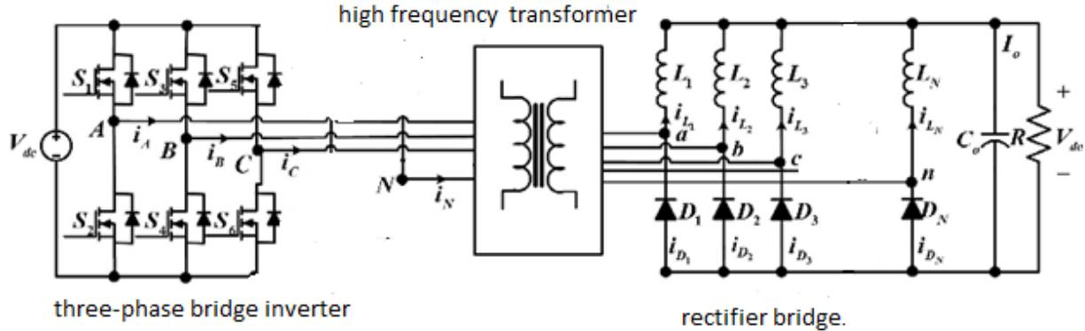
Fig. 1. Three-phase high frequency isolated DC-DC converter.
