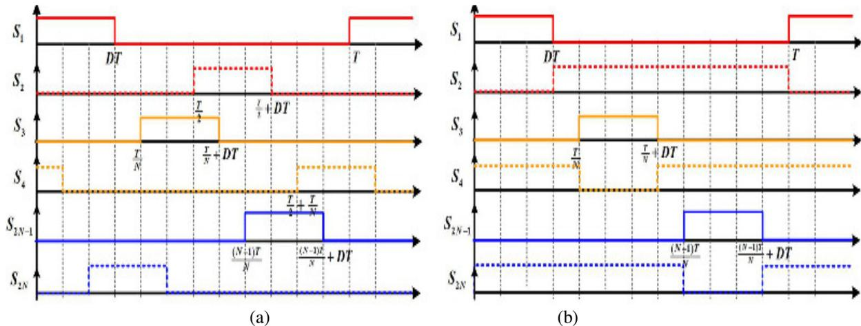
Fig. 2. Control methods: (a) symmetrical. (b) Asymmetrical.
