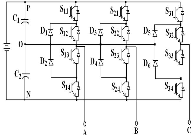
Fig no. 01 : Schematic diagram of three-level inverter
