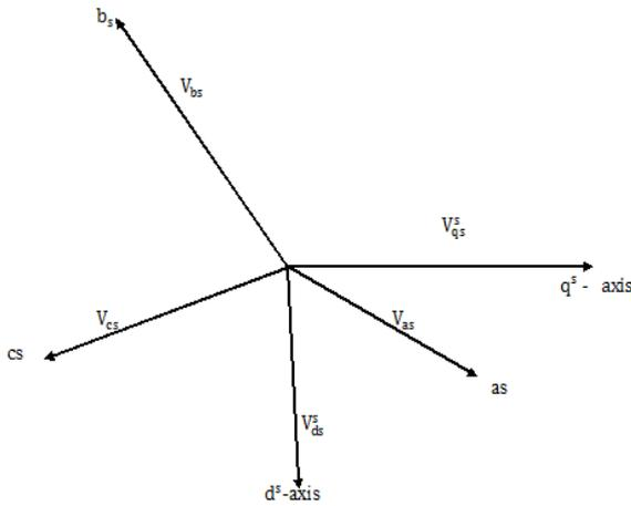
Fig. 2.1 Stationary Frame a-b-c to d<sup>s</sup>-q<sup>s</sup> Axes Transform motion
