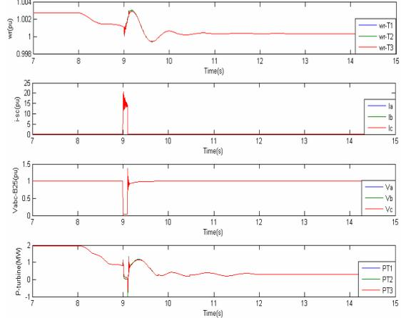
Fig. 17. LLLG fault results (decreasing wind speed)
