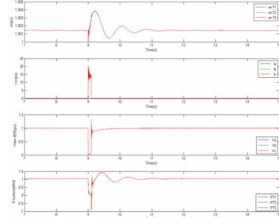
Figure 9. LLLG fault results (constant wind speed 7 m/s)
