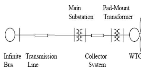
Figure 1. A typical network topology of a wind power plant
