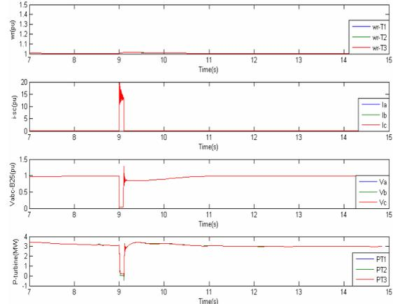
Fig. 12. LLLG fault results (constant wind speed 10 m/s)
