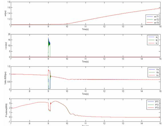
Figure 8. LLLG fault results (increasing wind speed)
