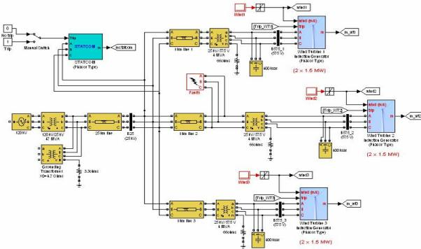
Figure 11. Matlab-Simulink model of the case study with STATCOM
