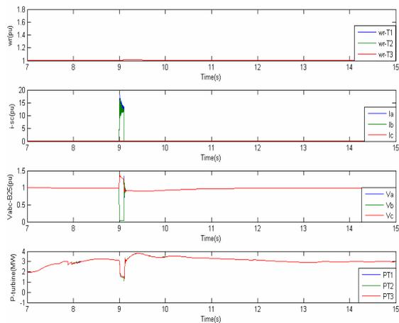
Fig. 15. LLLG fault results (increasing wind speed)
