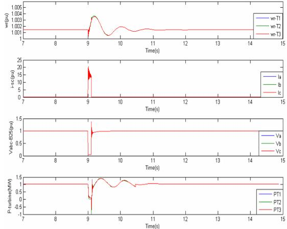
Fig. 16. LLLG fault results (constant wind speed 7 m/s)
