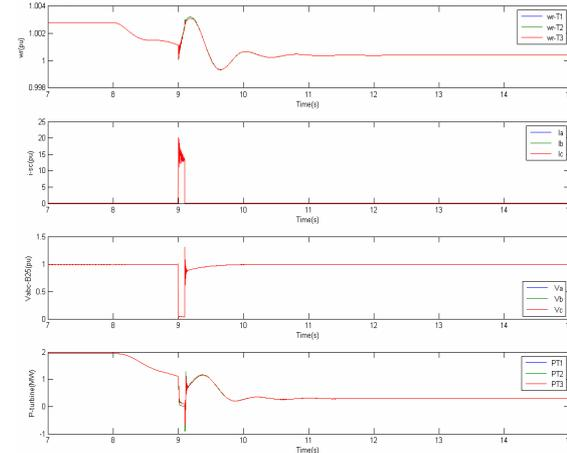
Figure 10. LLLG fault results (decreasing wind speed)
