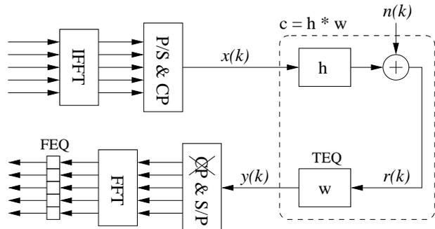
Figure 1: System model. (I)FFT: (inverse) fast Fourier transform, P/S: parallel to serial, CP: add cyclic prefix, xCP: remove cyclic prefix.
