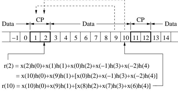
Figure 2: Illustration of the difference in the ISI at the received CP and at the end of the received symbol.  $x(i)$ ,  $h(i)$ , and  $r(i)$  are the transmitted data, channel, and received data, respectively.
