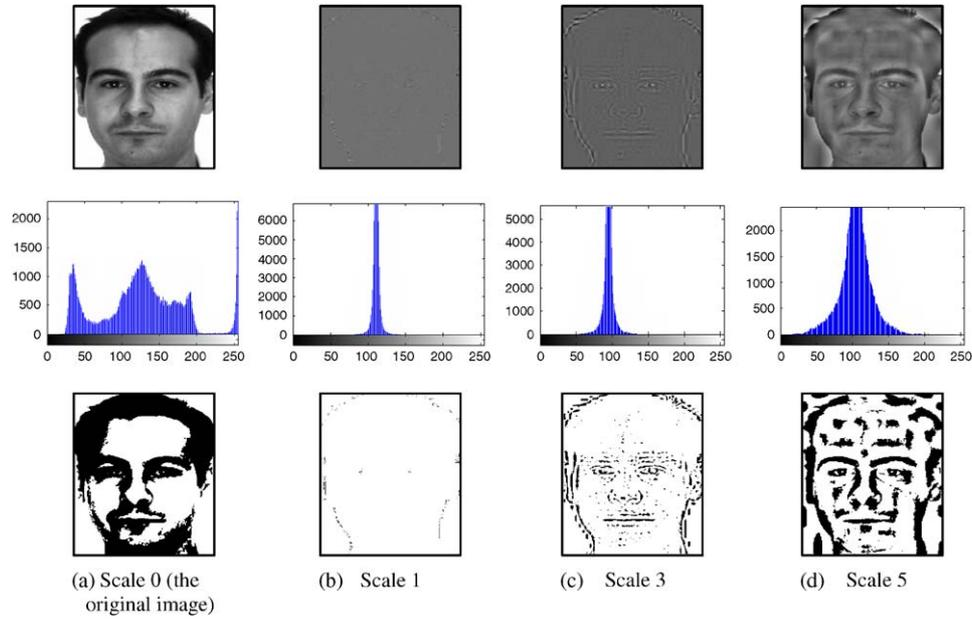
Fig. 2. Images reconstructed with high-frequency components at different scales, their histograms and binary edge images (from upper to lower).
