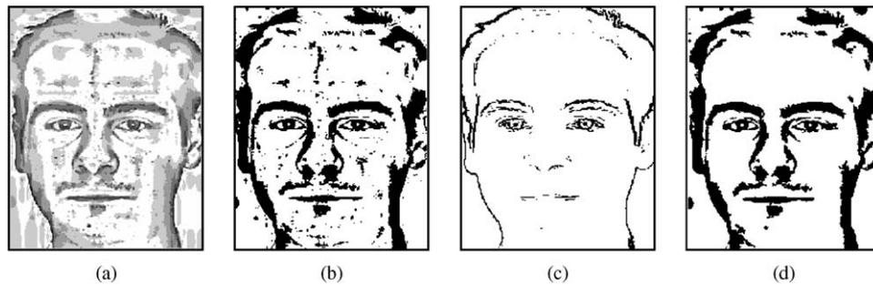
Fig. 3. Extraction of face edges. (a) The merged edge image, (b) BEI after binarization, (c) BEM, (d) BEI after noise removing.
