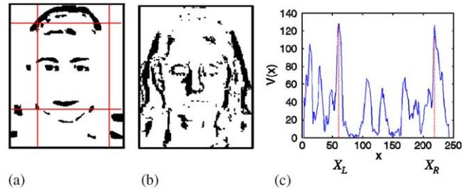
Fig. 7. Refinement of the face region. (a) BEI after the boundary pixel removing operation, (b) removed parts, (c) vertical projection of (b).
