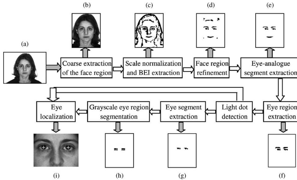
Fig. 1. Flowchart of our proposed eye detection method.
