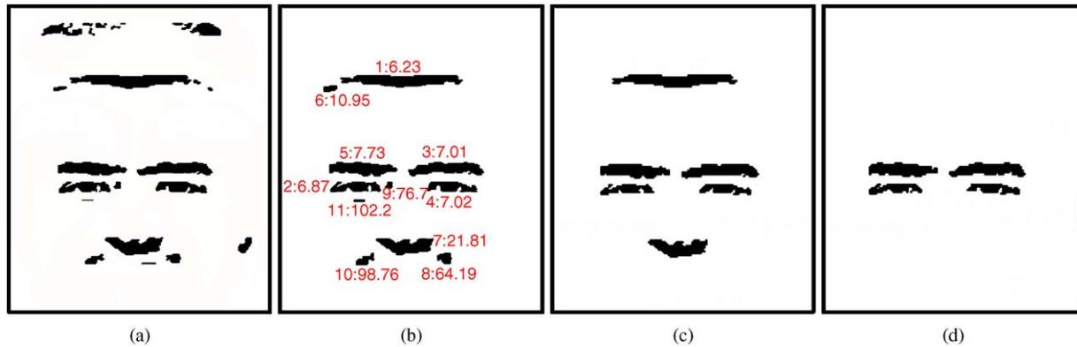
Fig. 8. Detection of eye region. (a) RBEI, (b) PESBEI, (c) EASBEI, and (d) ERBEI.
