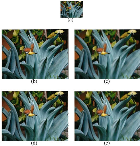
Figure 6. 3X magnification of the bird image: (a) input low-resolution image; (b) true high-resolution image; (c) median filtering; (d) cubic spline interpolation; (e) our method with training images shown in Figures 2(c) and (d).
