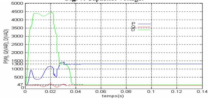
**Fig. 8.** Active, reactive and distortion powers.
