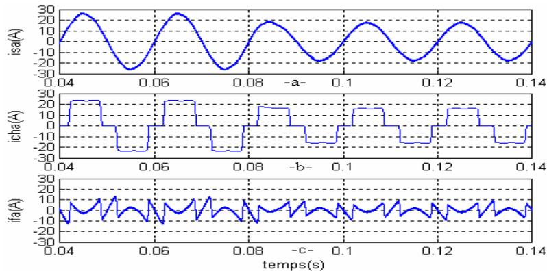
**Fig. 10.** (a) supply current; (b) load current; (c) compensating current waveform after harmonic compensation
