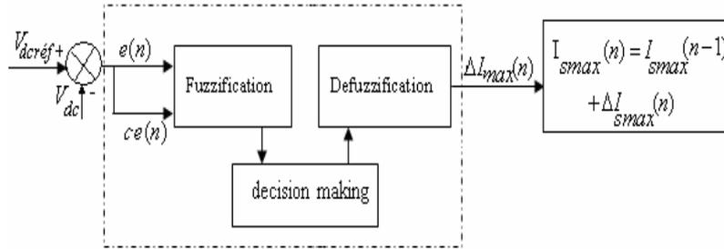
Fig. 3. Internal structure of fuzzy logic controller
