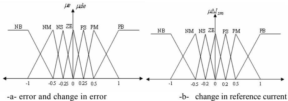
Fig. 4. Normalized triangular membership functions used in fuzzification.
