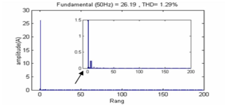
**Fig. 6.** Harmonics spectra of line-current
