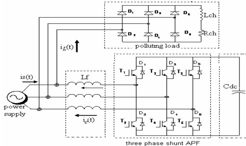
Fig. 1. Shunt active power filter topology.
