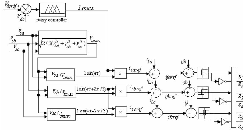
Fig. 2. Bloc diagram of direct current control
