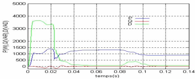
**Fig. 13.** Active, reactive and distorting powers
