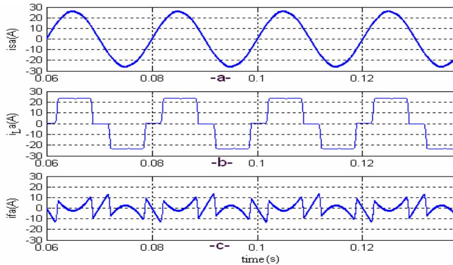
**Fig. 5.** (a) Supply current; (b) load current; (c) compensating current waveform after harmonic compensation
