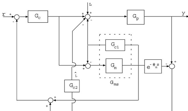
Fig. 1. The new Smith predictor structure.
