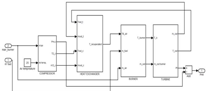
**Fig. 6.** Matlab/Simulink model of microturbine
