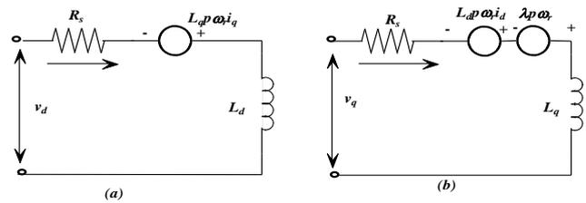
Fig. 2. d q-axis equivalent circuit of PMSM
