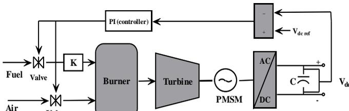
Fig. 3. Block diagram of MTG system controller
