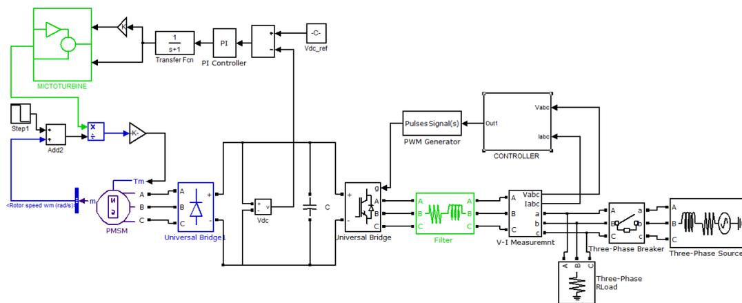
**Fig. 7.** Matlab/Simulink model of MTG system in connected grid/Islanding
