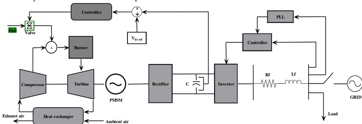
**Fig. 1. Microturbine generation (MTG) system**
