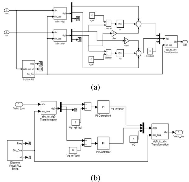
Fig. 4. (a). Line side converter control, grid connected, (b). Converter control, isolated mode
