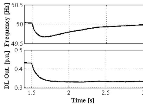
Fig. 6 – Frequency and DL output during load connection.
