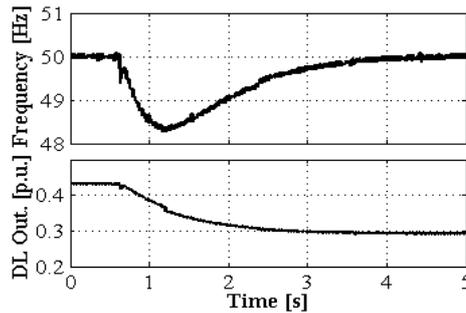
Fig. 9 – Frequency and DL output during load connection.
