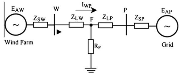
Fig. 2. Line diagram for phase A-to-ground fault [14].
