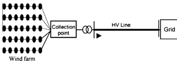
Fig. 1. Interconnection of wind farm to the grid [14].
