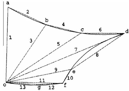
Fig. 5. Adaptive setting characteristic and topological trip-decision logic [6].
