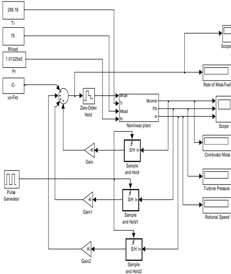
Fig .3 closed loop block diagram of the nonlinear system by using MATLAB Simulink
