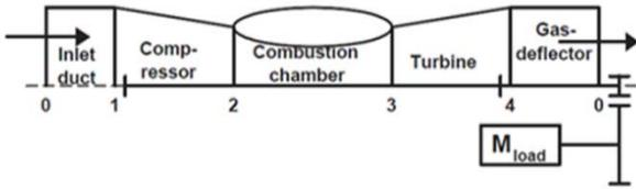
Fig.1 the main parts of the gas turbine
