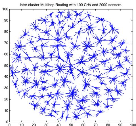
Fig. 1. Transmissions in the network with inter-cluster multihop routing when the BS at the center
