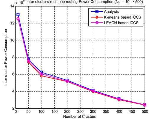
Fig. 7. Inter-cluster power consumption when BS at the center in a circle sensing area
