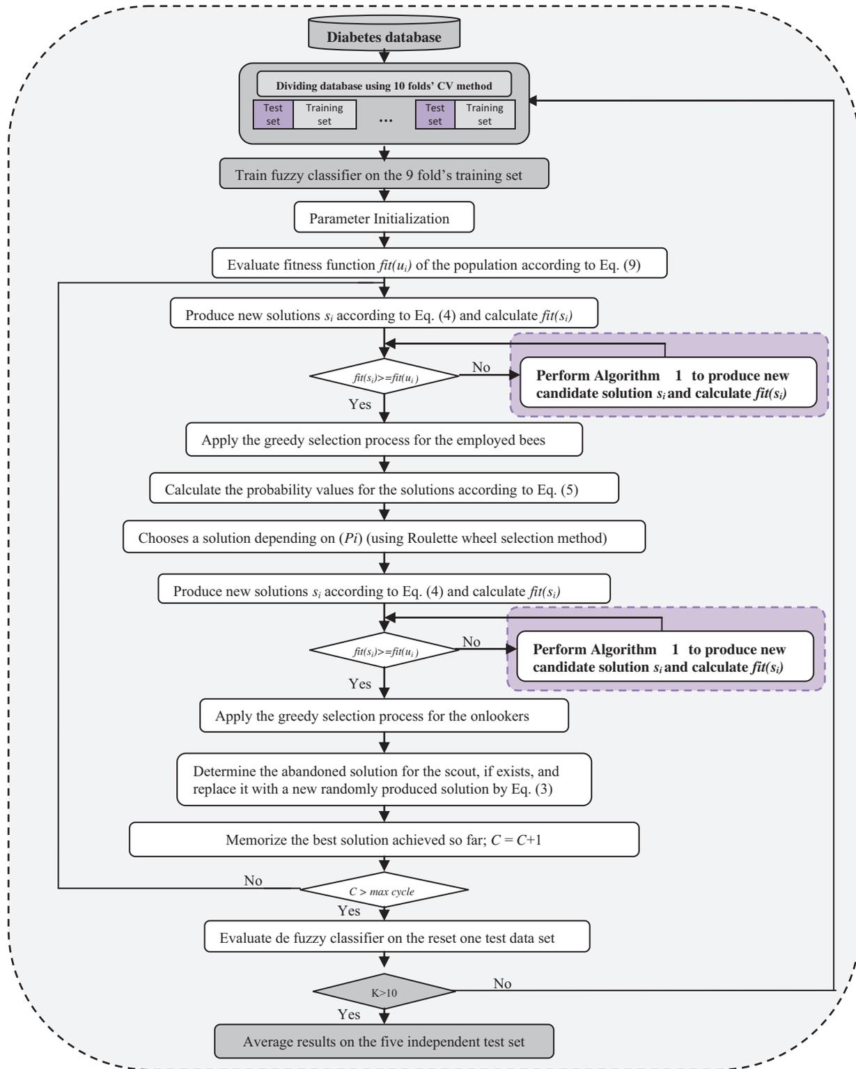
Fig. 4 – The flow chart of the proposed algorithm.
