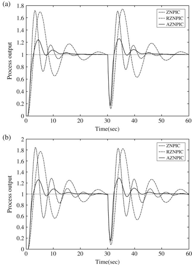
Fig. 7. Responses of the third-order linear process in (14) with (a)  $L = 0.4$  s and (b)  $L = 0.5$  s.
