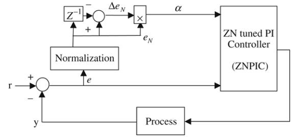
Fig. 1. Block diagram of the proposed AZNPIC.
