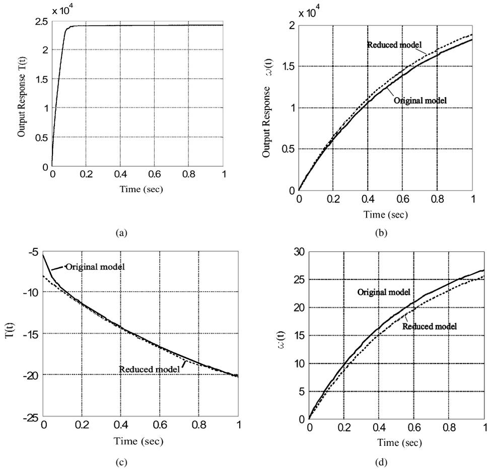
Fig. 2. (a) Temperature variation following a unit step change on the fuel flow. (b) Speed variation following a unit step change on the fuel flow. (c) Temperature variation following a unit step change on the nozzle area. (d) Speed variation following a unit step change on nozzle area.
