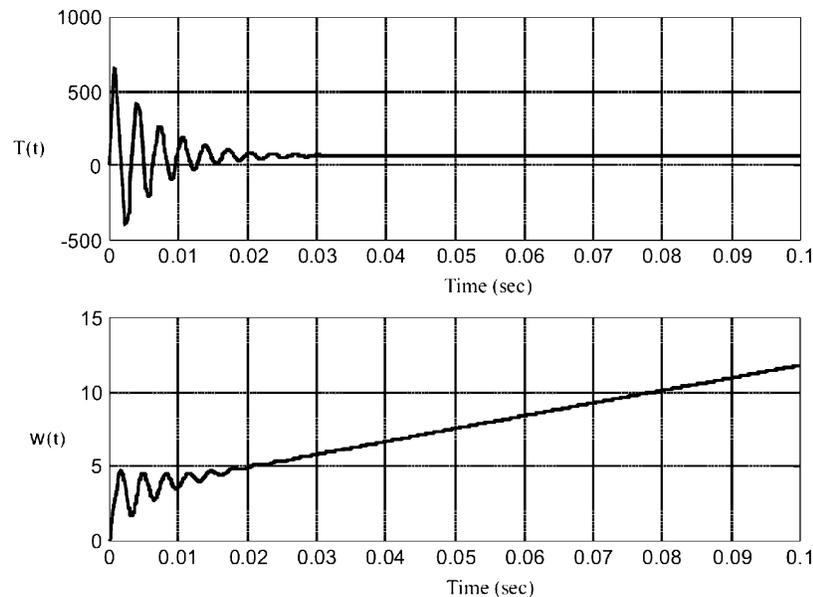
Fig. 4. Inner closed loop system response following a step change on  $r(t)$ .
