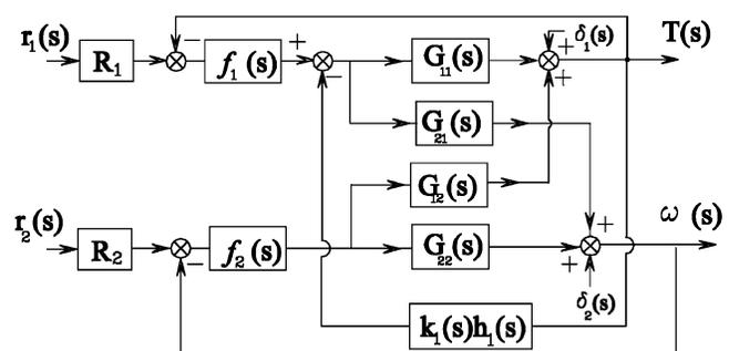
Fig. 6. Block diagram of final closed loop system for implementation purposes.
