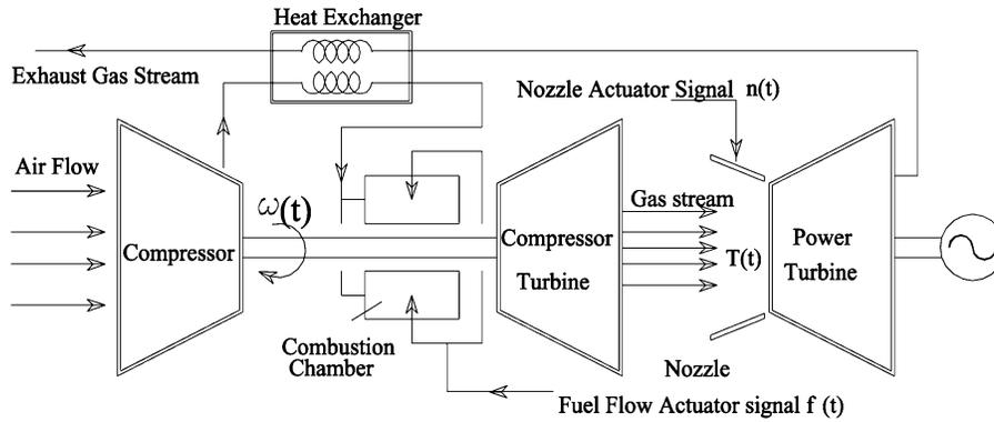
Fig. 1. Arrangement of automotive gas turbine.
