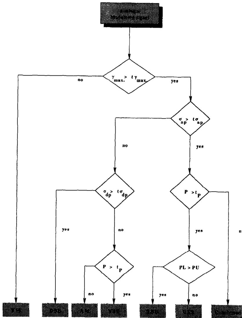
Fig. 1. Functional flowchart for automatic recognition of analogue modulations.
